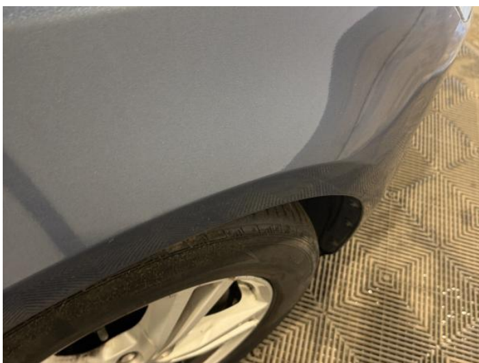
19: Wing osf Dented Between 10mm + 30mm
