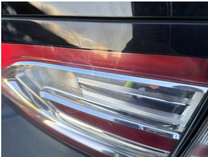
23: Lamp osr Broken Replace
