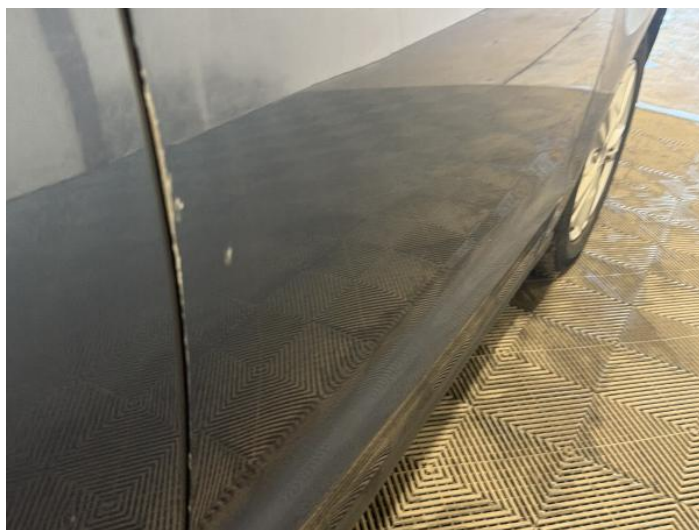
18: Door osf Scratched Over 25mm Thru Paint
