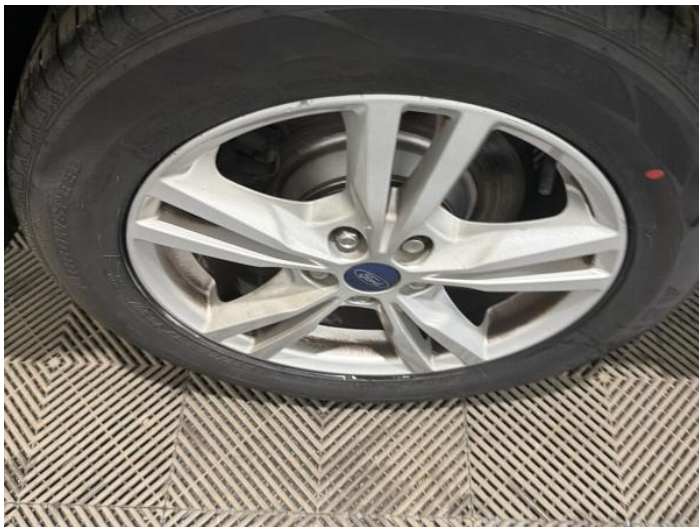
15: Wheel osr Scratched Up To 50mm
