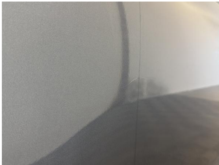
16: Door osr Scratched UpTo 25mm Thru Paint
