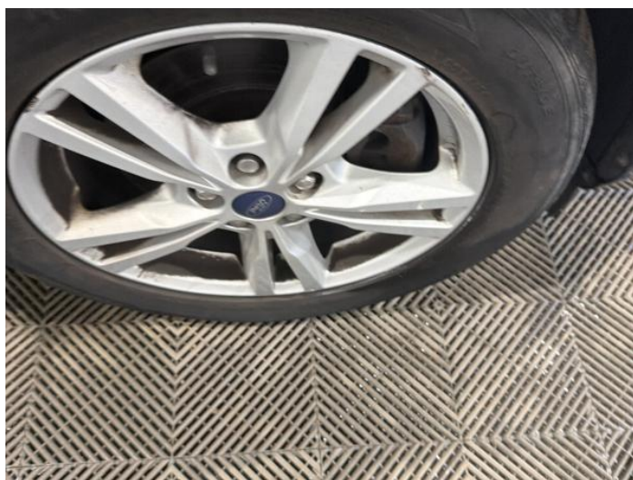
20: Wheel osf Scratched Over 50mm
