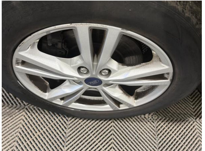
4: Wheel nsf Scratched Up To 50mm
