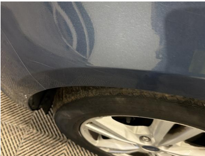
5: Wing nsf Scratched Up To 25mm Thru Paint
