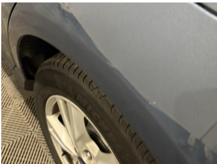
11: Qtr Panel nsr Dented With Paint Damage
