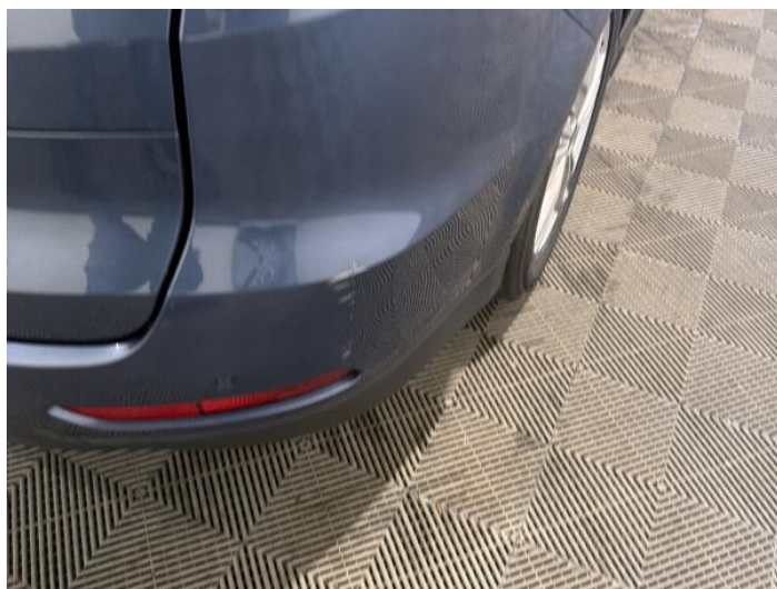
12: Bumper Rear Scratched Over 100mm Thru Paint
