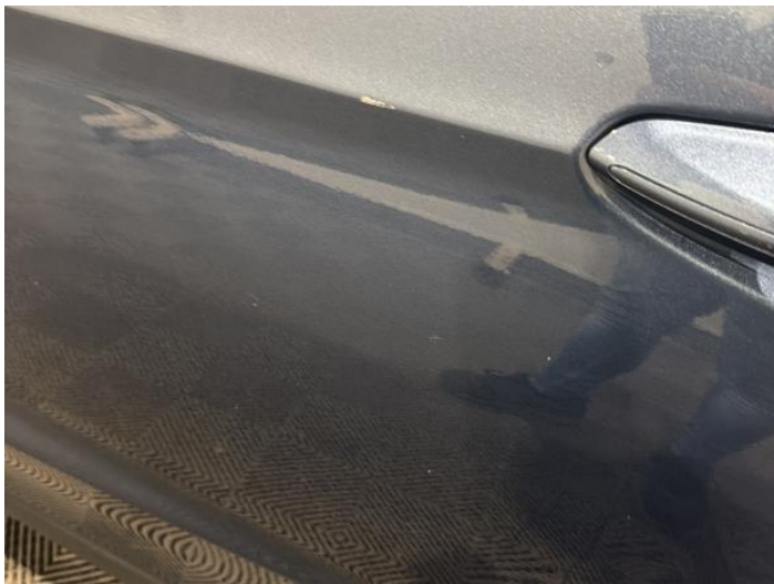
9: Door nsr Scratched Over 25mm Thru Paint
