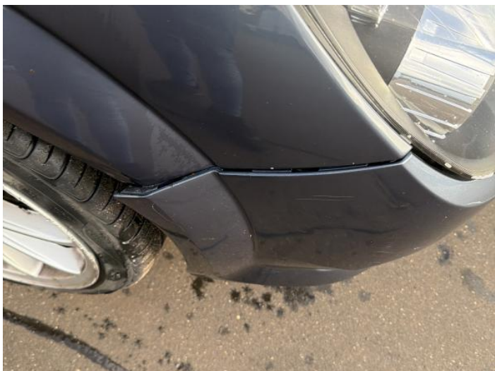
3: Bumper Front Insecure Action Required
