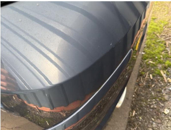
11: Bumper Rear Poor Previous Repair Poor Paint
