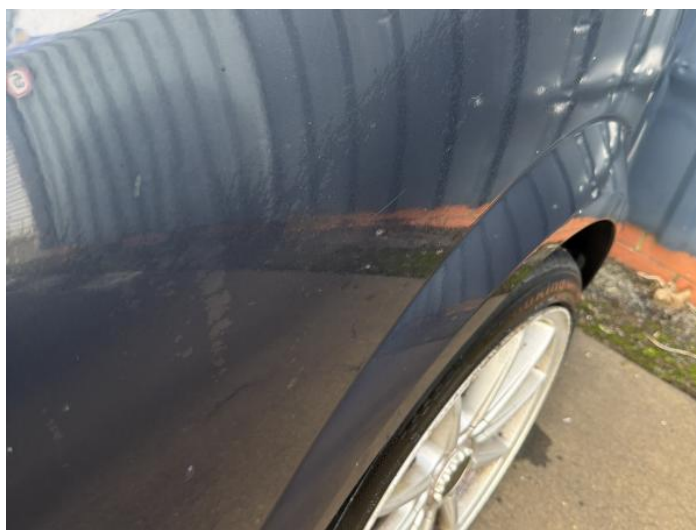
8: Qtr Panel nsr Dented With Paint Damage
