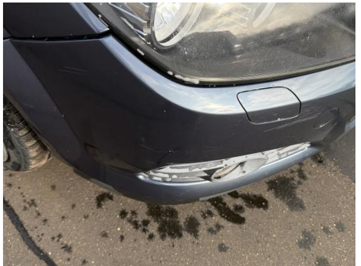
2: Bumper Front Scratched Over 100mm Thru Paint
