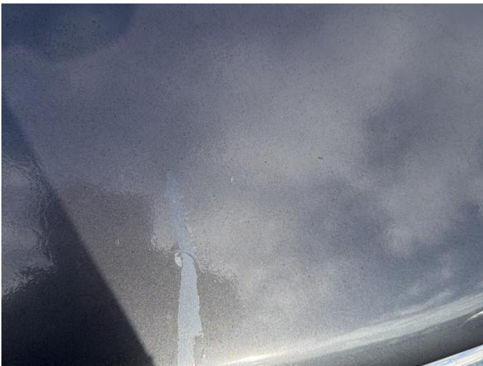
1: Bonnet Poor Previous Repair Paint Flake
