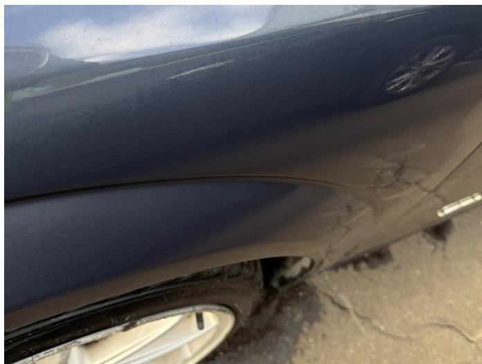
4: Wing nsf Dented Over 2 UpTo 10mm
