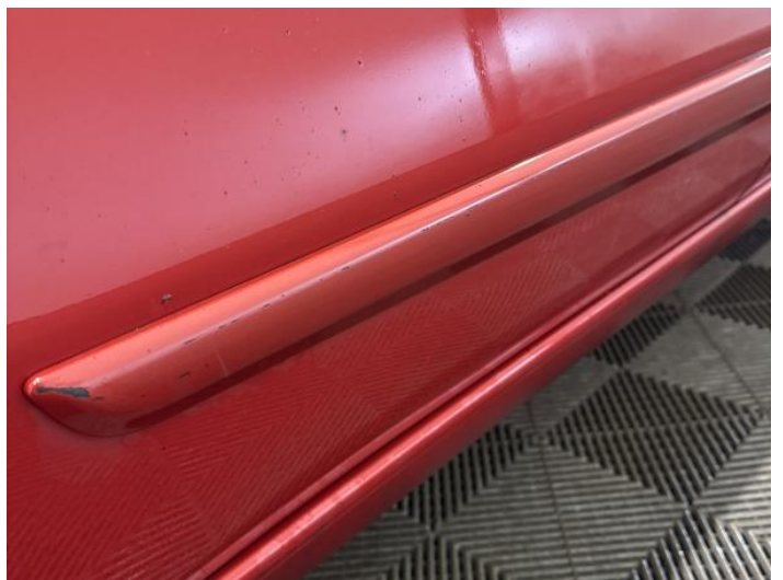
14: Door Moulding osr Scratched (Painted) Over 25mm Thru Paint
