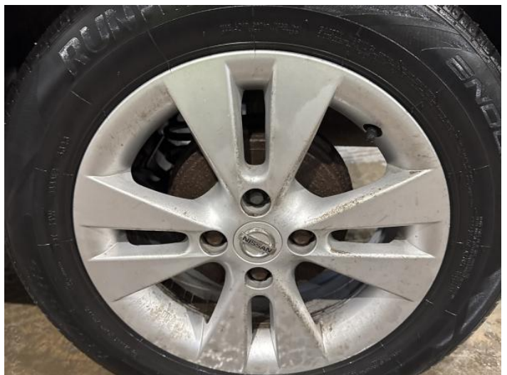
8: Wheel nsr Scratched Up To 50mm
