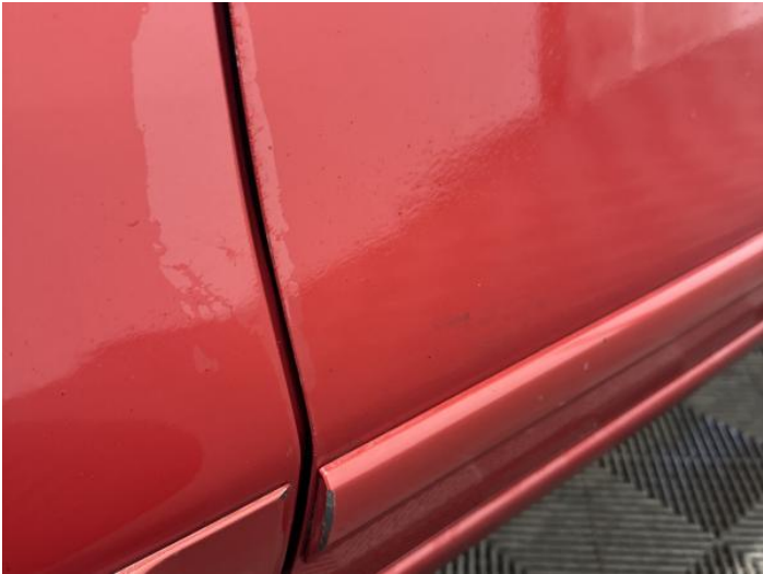
15: Door osf Chipped Edge Chip
