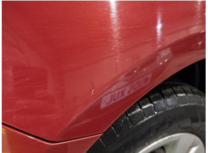
4: Wing nsf Scratched Up To 25mm Thru Paint
