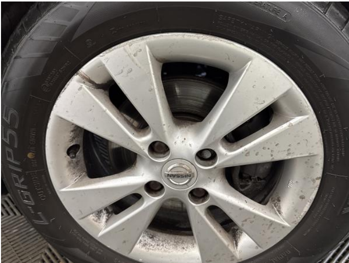
17: Wheel osf Scratched Over 50mm
