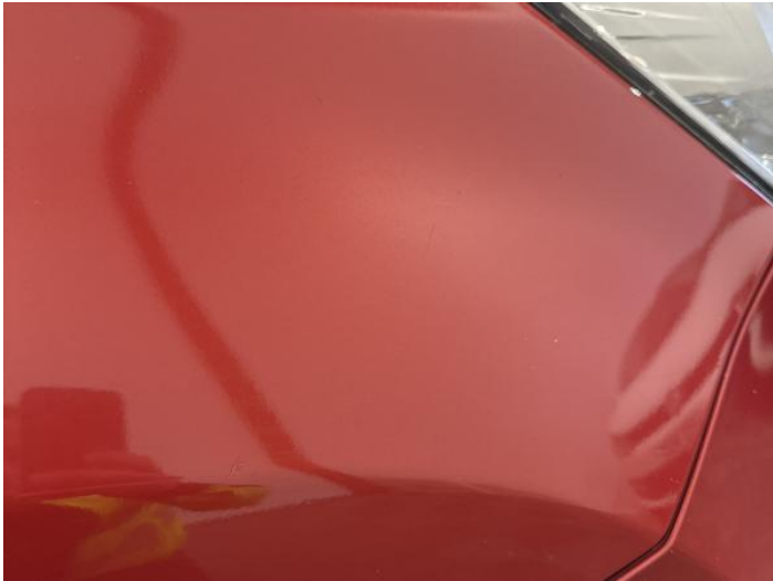
16: Wing osf Poor Previous Repair Poor Paint
