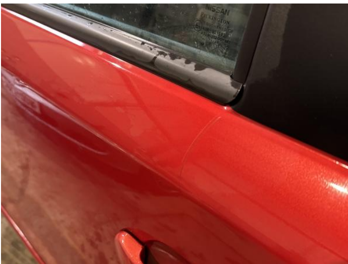
7: Door nsr Scratched Over 25mm Thru Paint
