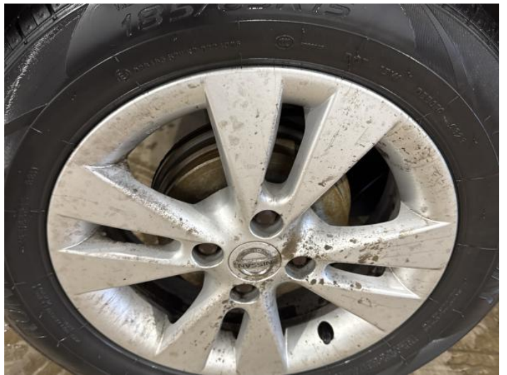
12: Wheel osr Scratched Up To 50mm
