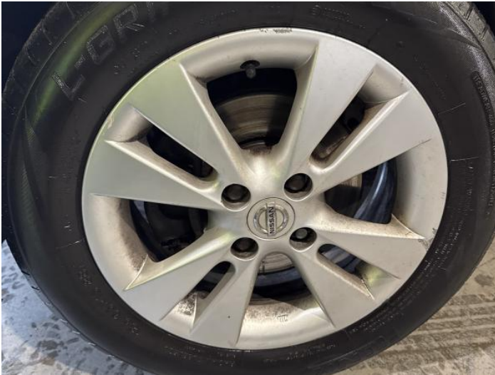
3: Wheel nsf Scratched Up To 50mm
