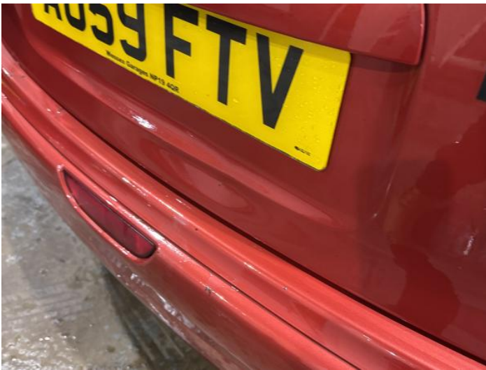
11: Tailgate Dented Over 30mm
