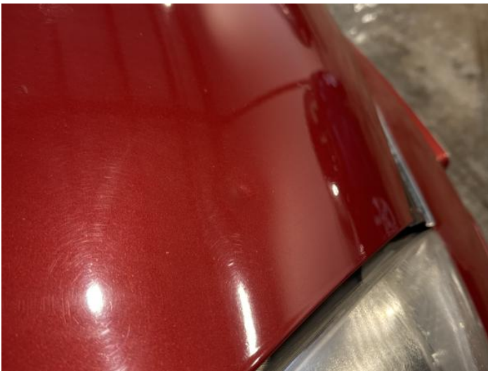
1: Bonnet Dented With Paint Damage
