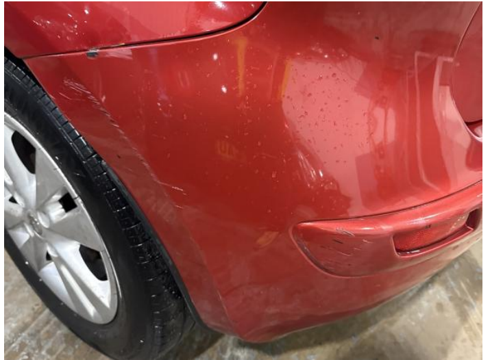
10: Bumper Rear Scratched Over 100mm Thru Paint
