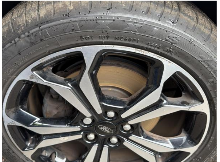
16: Wheel nsf Scratched Over 50mm
