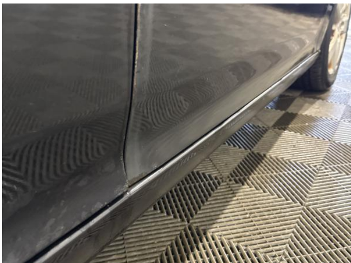
21: Door osf Dented Over 30mm
