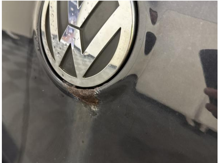
16: Tailgate Rusted Over 5mm
