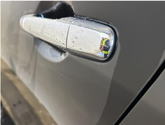
17: Door nsr Scratched Over 25mm Thru Paint
