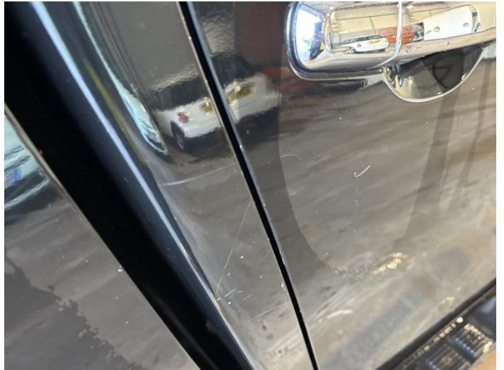
10: C Post os Scratched Over 25mm Thru Paint
