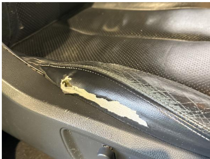
2: Seat Base Cover osf Holed Over 3mm
