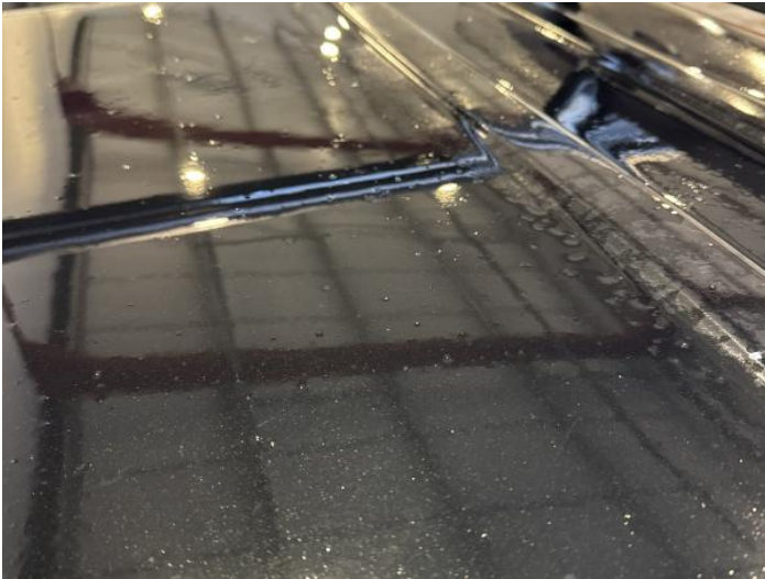
15: Roof Dented Over 30mm
