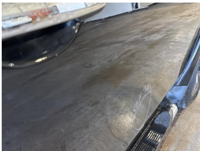
8: Door osf Dented Between 10mm + 30mm
