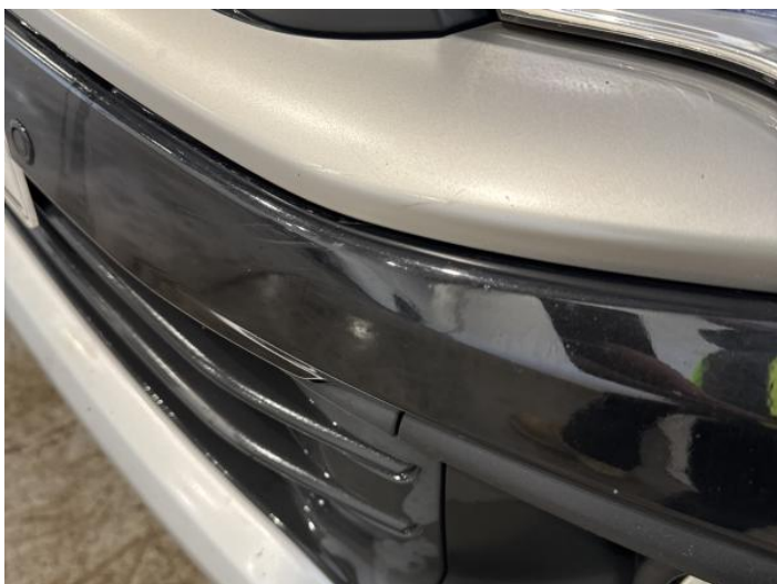
5: Bumper Front Chipped Multiple Chips
