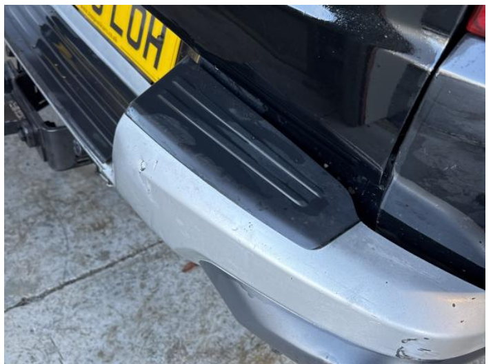
14: Bumper Rear Dented With Paint Damage
