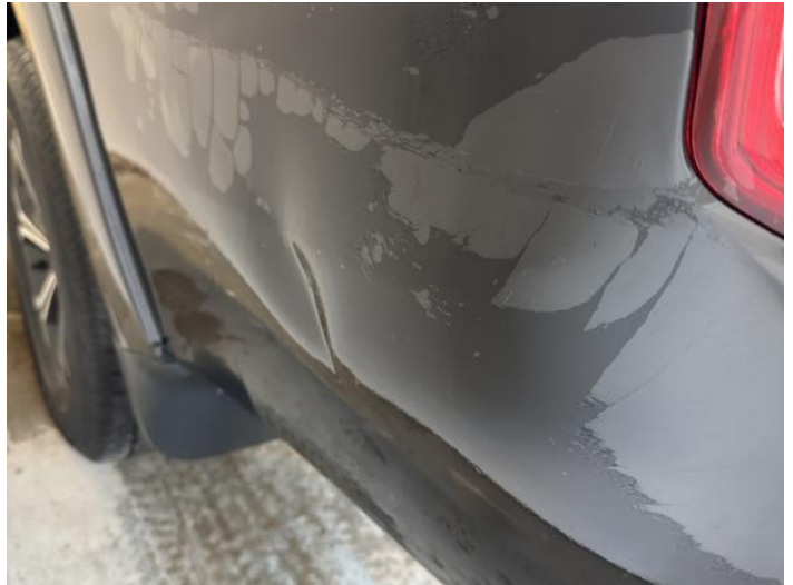
16: Qtr Panel nsr Dented Over 30mm
