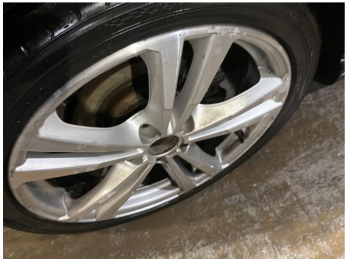
6: Wheel osr Scratched Over 50mm
