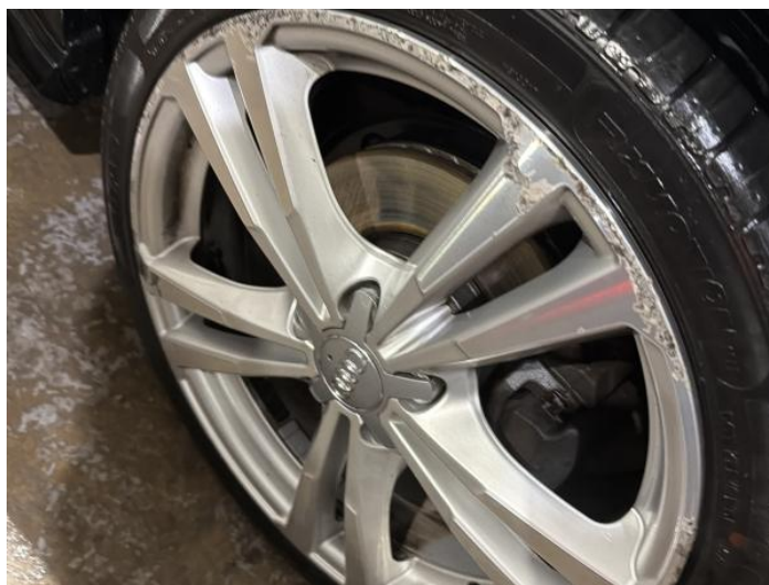
12: Wheel osf Scratched Over 50mm
