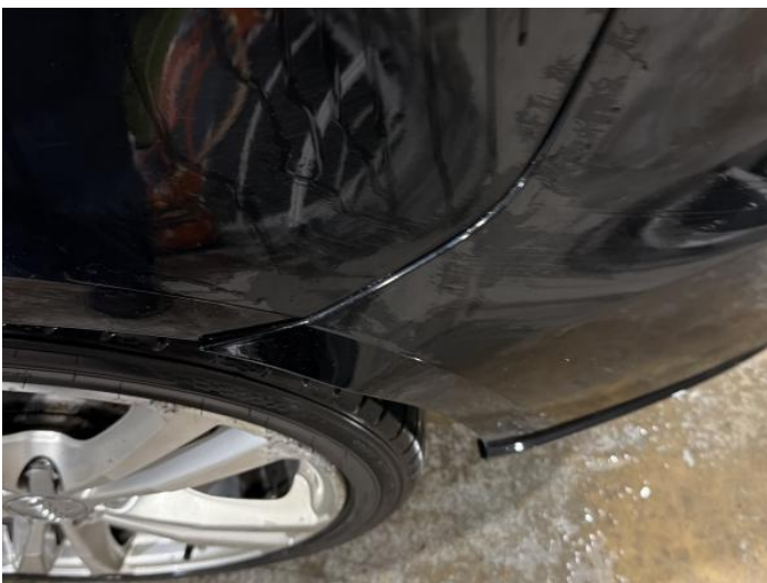
25: Bumper Rear Insecure Action Required
