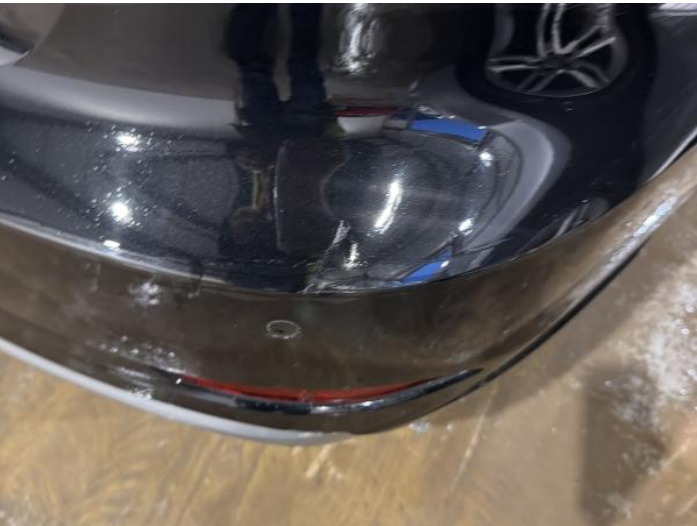
1: Bumper Rear Scratched 25 to 100mm Thru Paint
