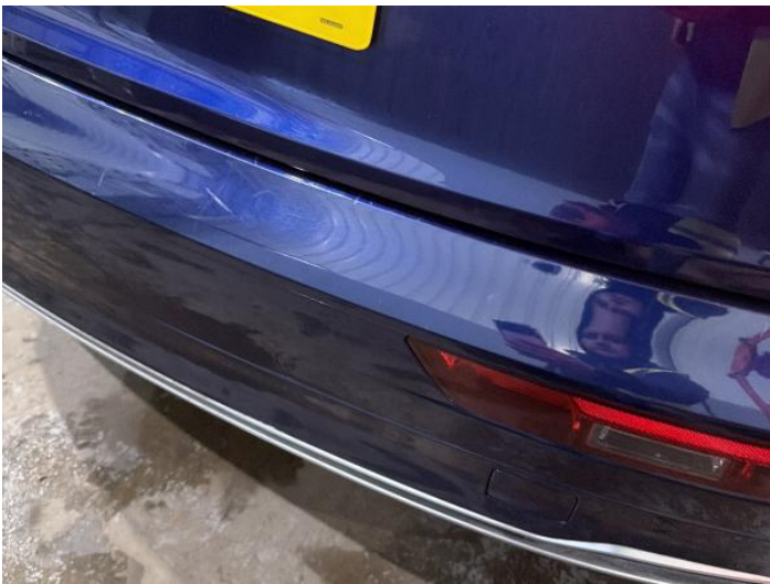
11: Bumper Rear Scratched 25 to 100mm Thru Paint
