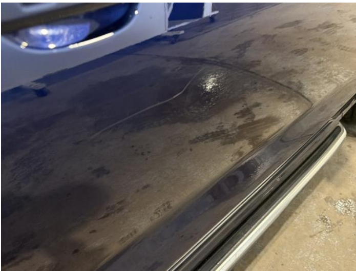
17: Door osf Scratched Over 25mm Thru Paint
