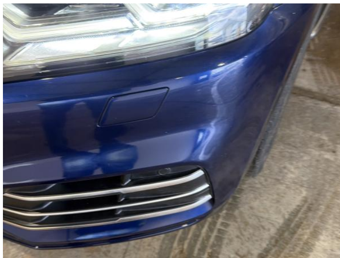
2: Bumper Front Scratched 25 to 100mm Thru Paint
