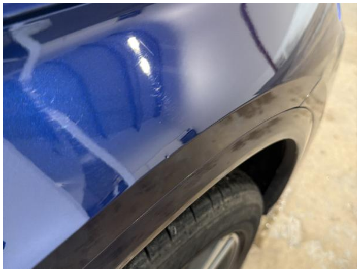
18: Wing osf Dented Between 10mm + 30mm
