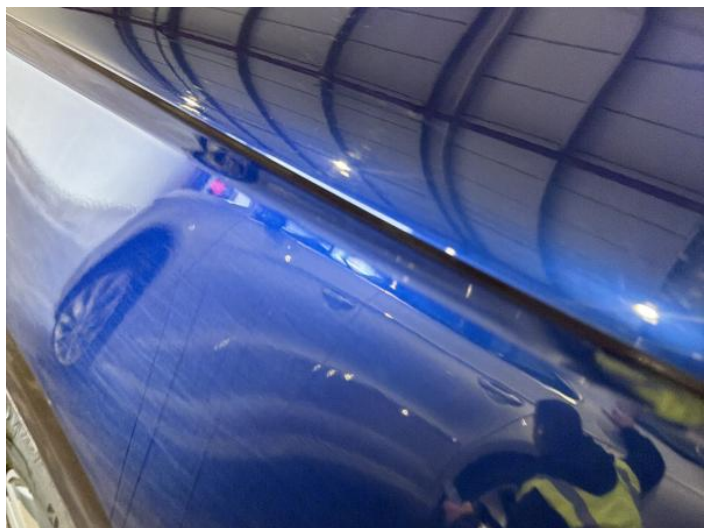
8: Qtr Panel nsr Dented Over 2 UpTo 10mm
