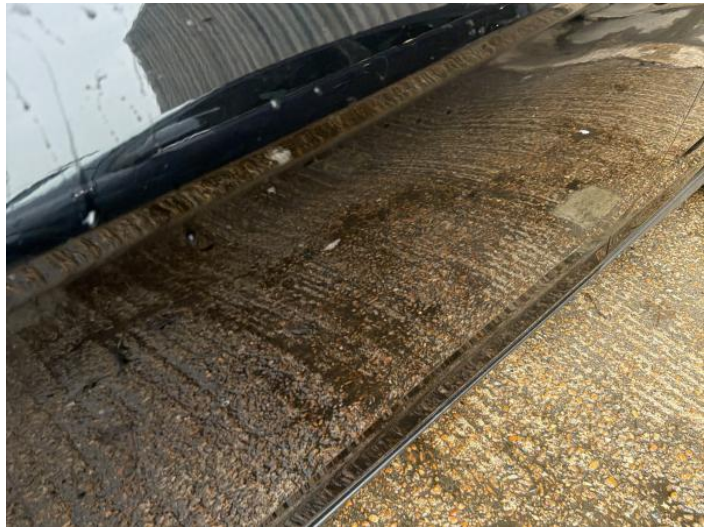
18: Door nsf Chipped Multiple Chips
