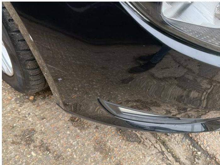
12: Bumper Front Scratched 25 to 100mm Thru Paint
