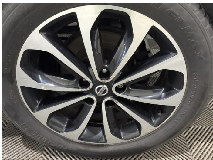
7: Wheel osr Scratched Over 50mm
