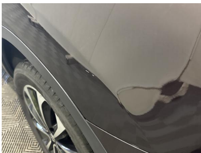
8: Qtr Panel nsr Scratched UpTo 25mm Thru Paint
