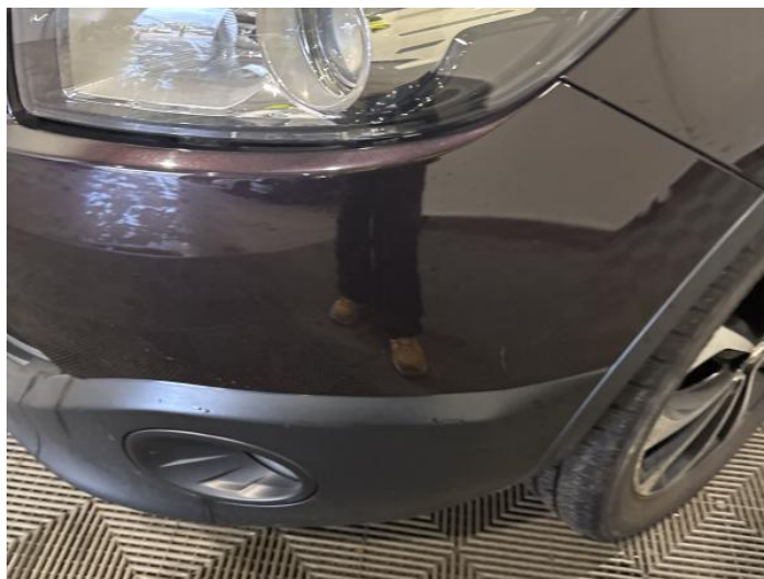
2: Bumper Front Scratched 25 to 100mm Thru Paint
