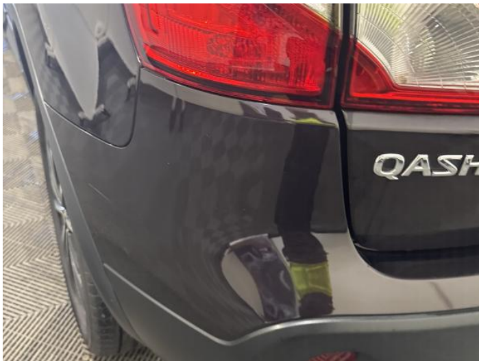
9: Bumper Rear Scratched Over 100mm Thru Paint
