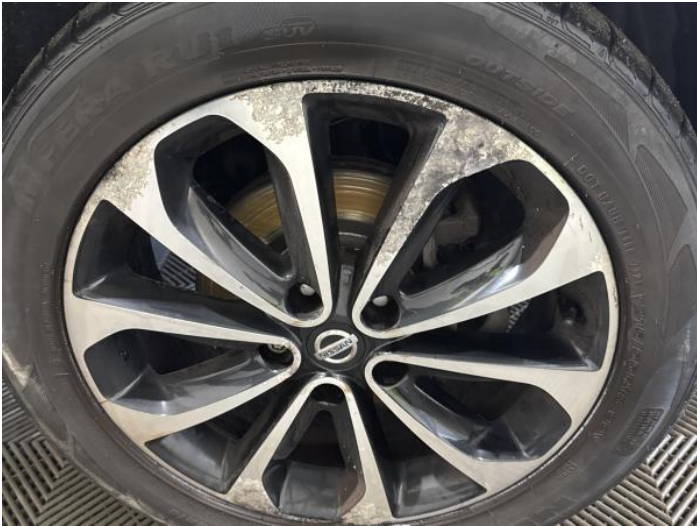
15: Wheel osf Scratched Over 50mm
