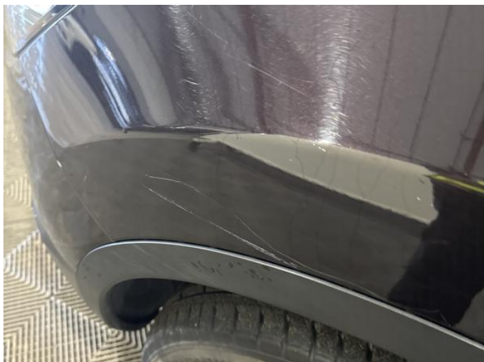
3: Wing nsf Scratched Over 25mm Thru Paint
