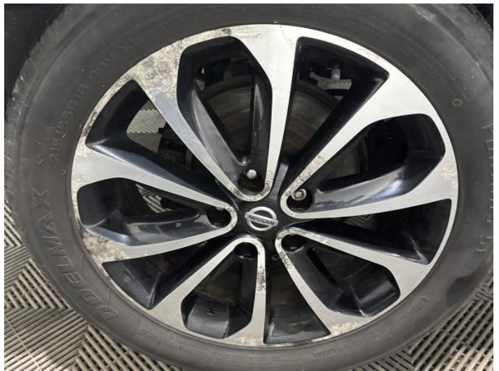
12: Wheel osr Scratched Over 50mm
