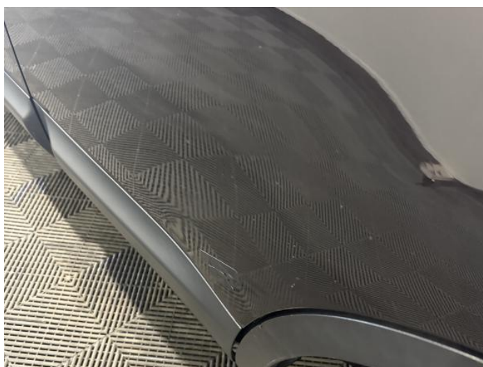
6: Door nsr Scratched Over 25mm Thru Paint
