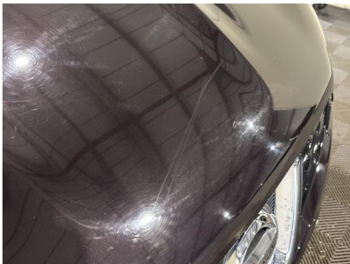
1: Bonnet Scratched Over 25mm Thru Paint
