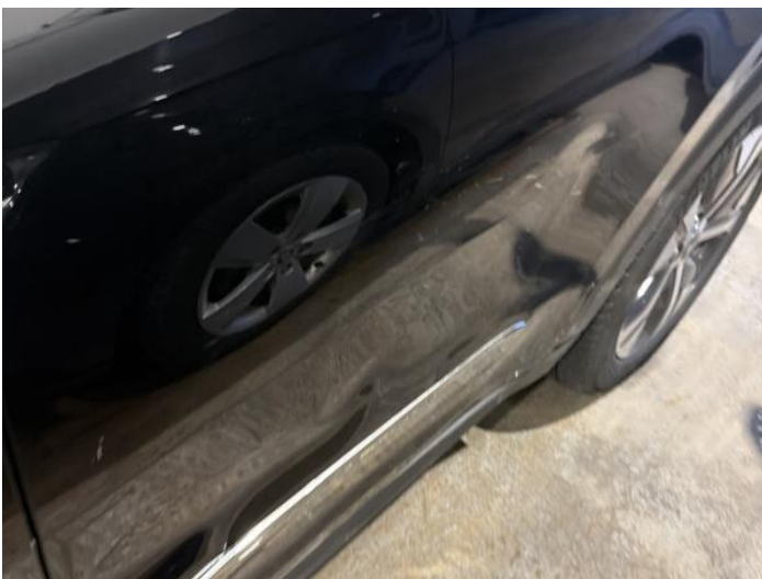
19: Door nsr Dented With Paint Damage
