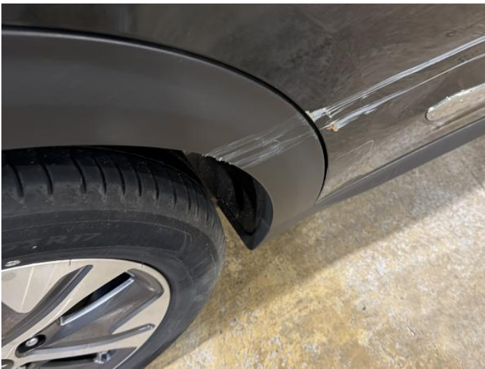
5: Qtr Panel Arch Extension os Scuffed (Unpainted) Over 100mm
