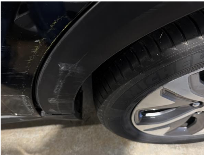
23: Qtr Panel Arch Extension ns Scuffed (Unpainted) Over 100mm
