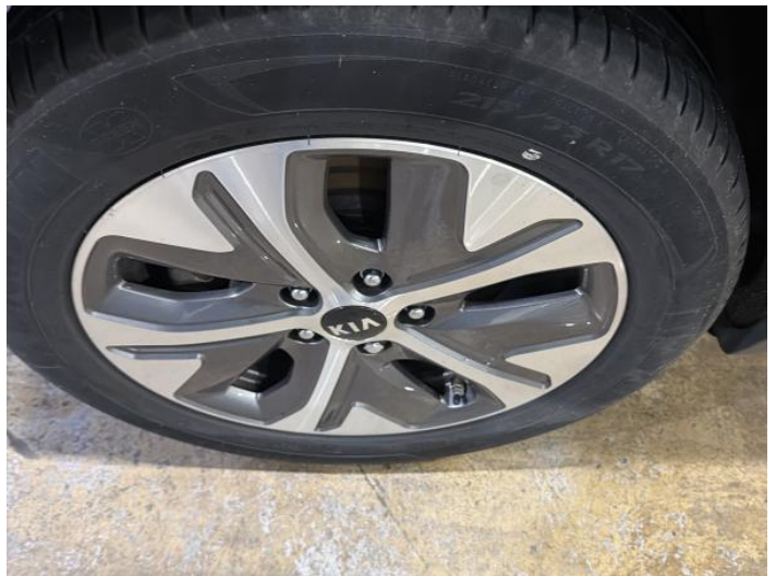
6: Wheel osr Scratched Up To 50mm
