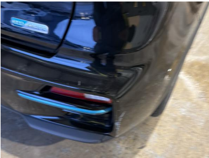
1: Bumper Rear Scratched Over 100mm Thru Paint
