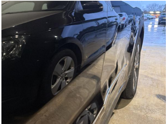
18: Door nsf Dented Over 30mm
