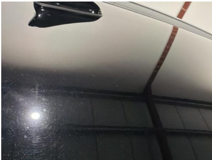
9: Roof Dented Hail - Moderate
