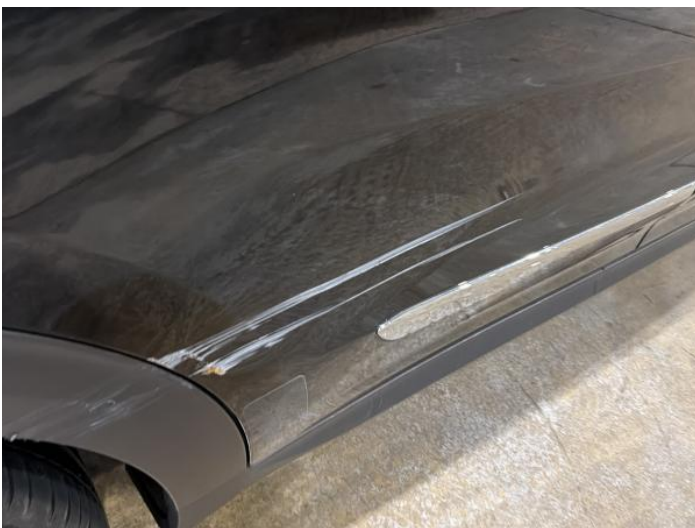
7: Door osr Dented With Paint Damage
