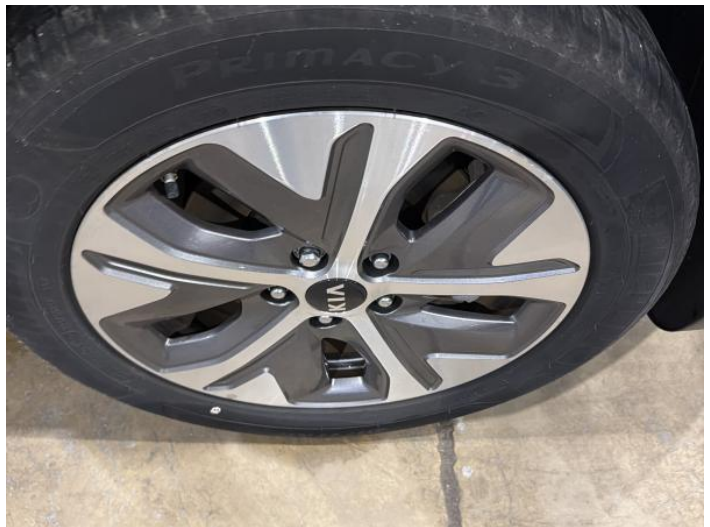
12: Wheel osr Scratched Up To 50mm
