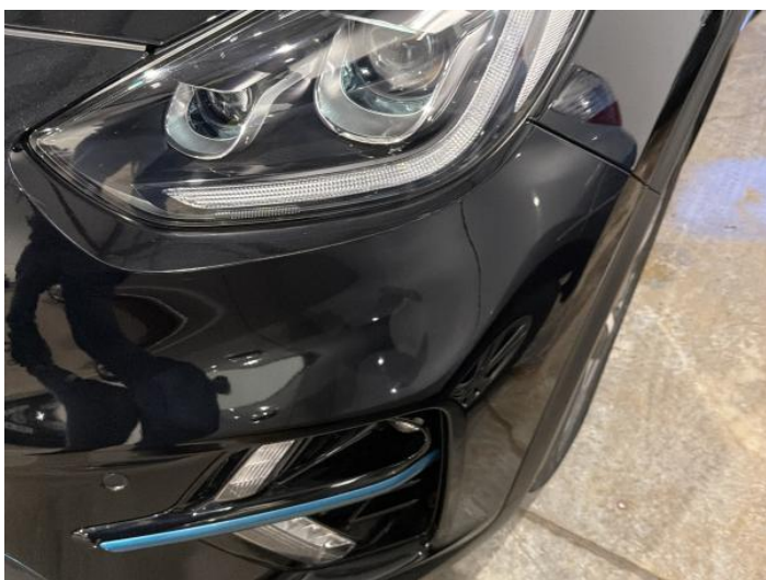
13: Bumper Front Scratched 25 to 100mm Thru Paint
