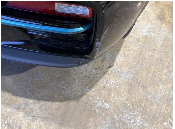
2: Bumper Rear Moulding Broken Replace
