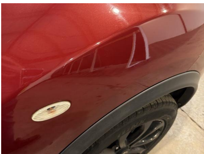
19: Wing osf Scratched Over 25mm Thru Paint
