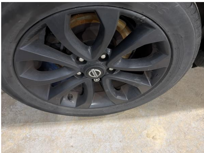
15: Wheel osr Scratched Over 50mm
