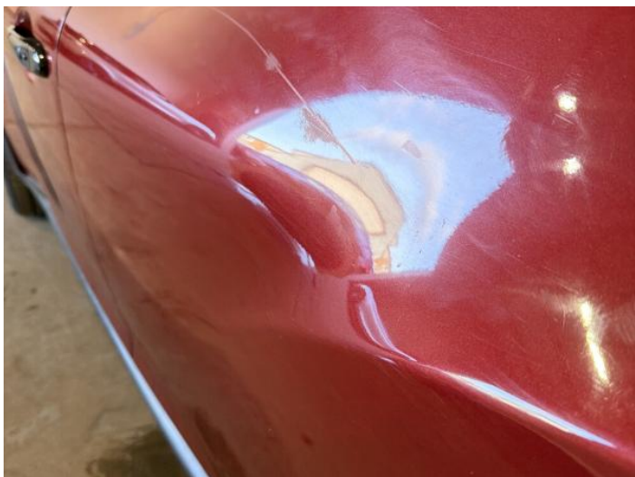
9: Door nsr Dented With Paint Damage
