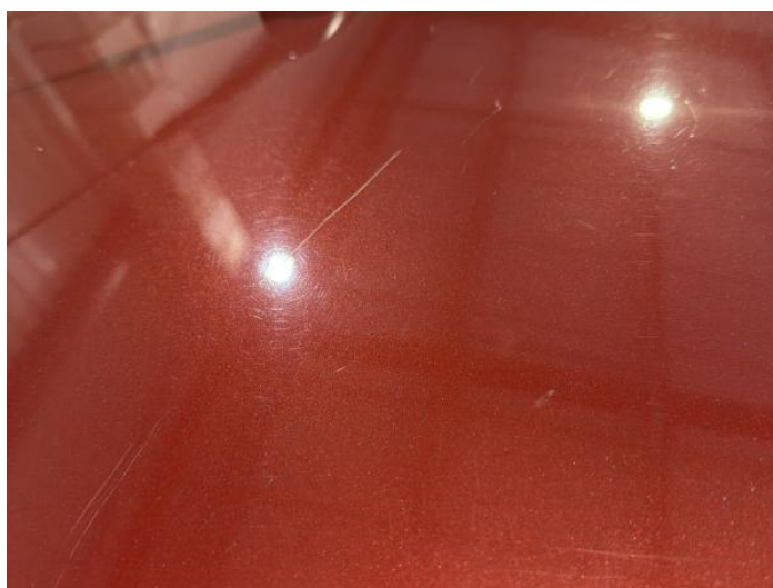
18: Roof Scratched Over 25mm Thru Paint
