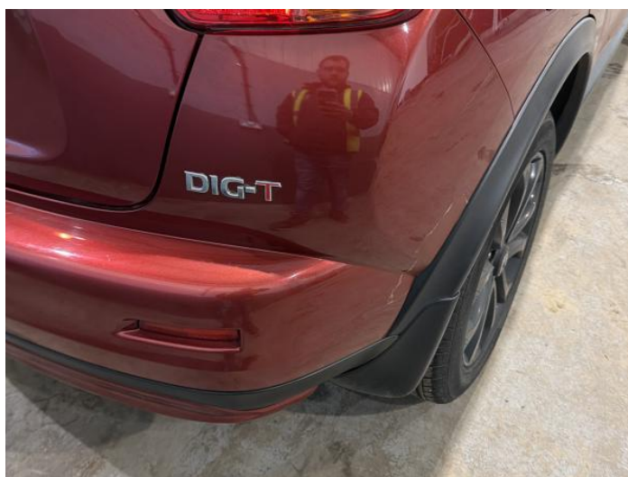
12: Bumper Rear Scratched Over 100mm Thru Paint
