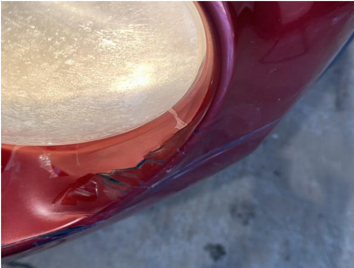
3: Bumper Front Cracked UpTo 25mm
