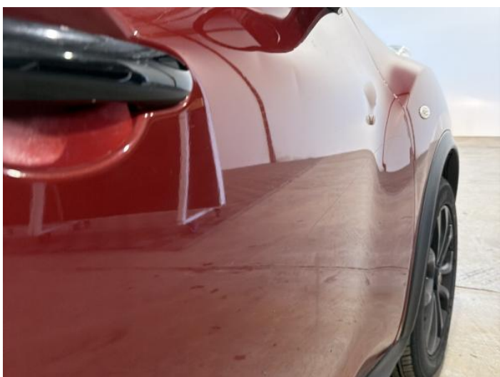
17: Door osf Dented Over 30mm
