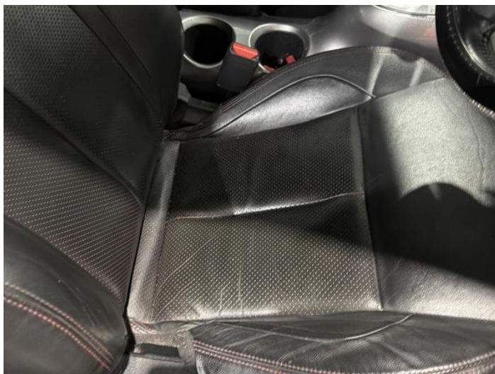
1: Seat Base Cover osf Scuffed Over 25mm
