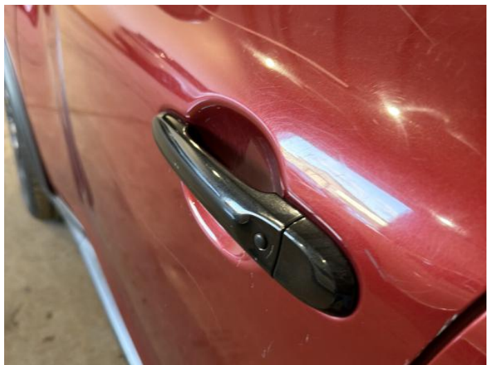
8: Door nsf Dented With Paint Damage
