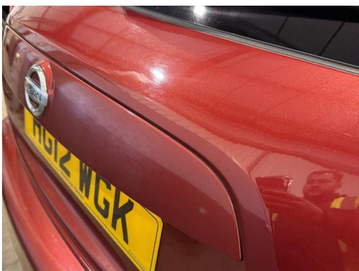
13: Boot Lid Dented Over 2 UpTo 10mm
