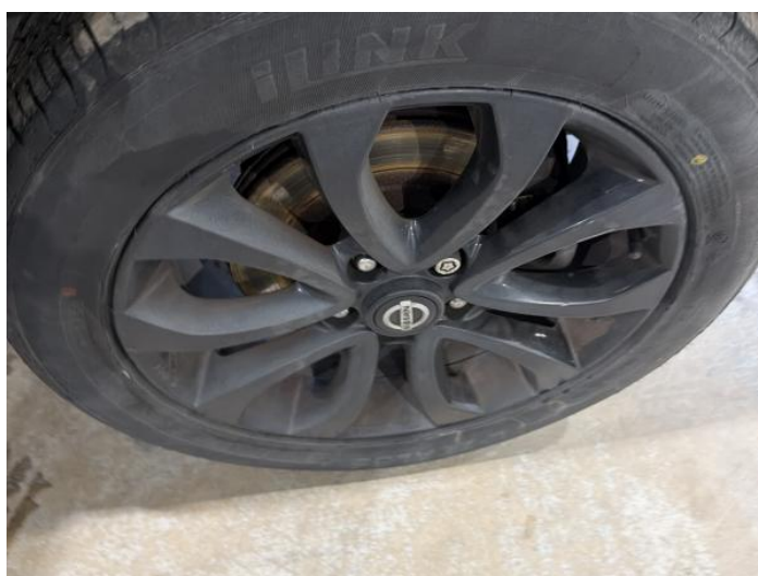
20: Wheel osf Scratched Over 50mm
