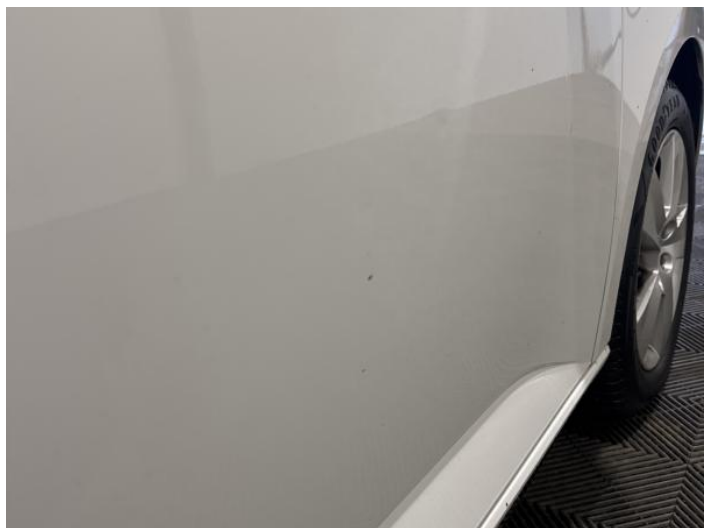
8: Door osf Dented Over 30mm
