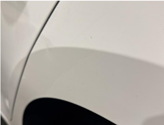
5: Qtr Panel nsr Dented Between 10mm + 30mm
