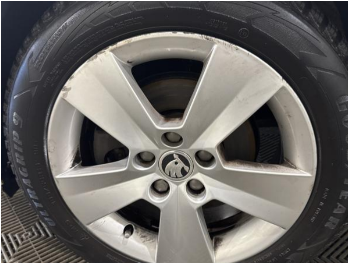
3: Wheel nsf Scratched Over 50mm
