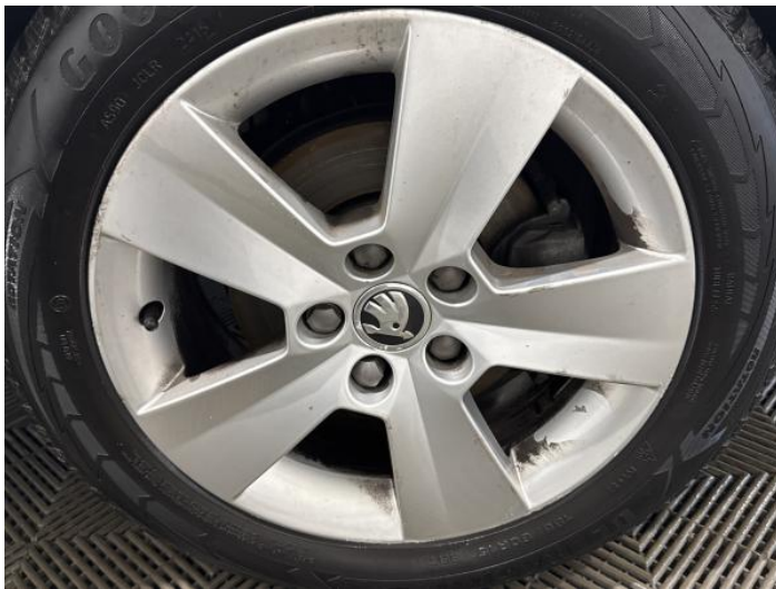
9: Wheel osf Scratched Over 50mm
