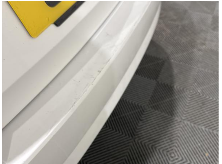
6: Bumper Rear Scratched 25 to 100mm Thru Paint
