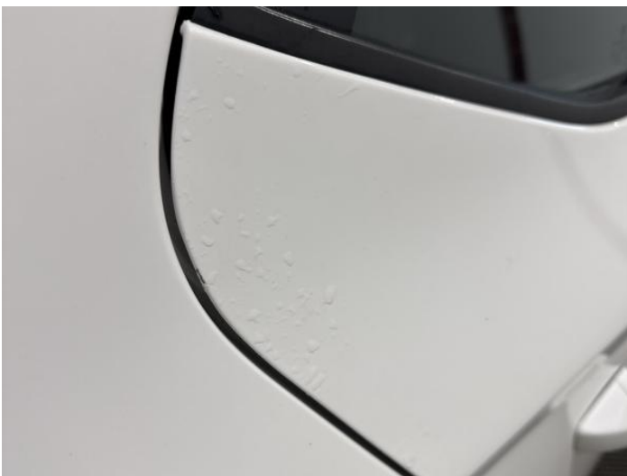
7: Door osr Chipped Edge Chip
