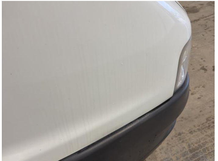
12: Wing osf Poor Previous Repair Poor Paint
