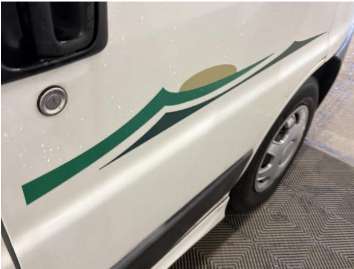
11: Door osf Poor Previous Repair Poor Paint
