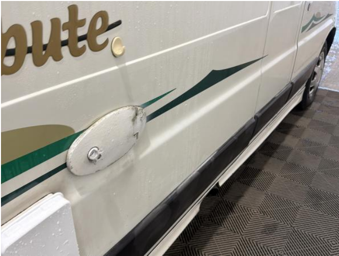
9: Door osr Poor Previous Repair Poor Paint
