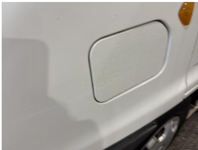
2: Wing nsf Poor Previous Repair Poor Paint
