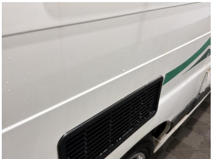
8: Qtr Panel osr Dented With Paint Damage
