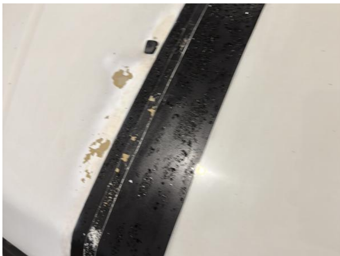
1: Bonnet Poor Previous Repair Paint Flake
