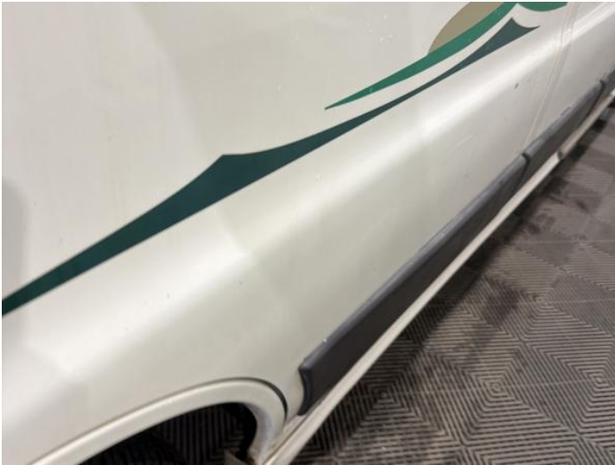
3: Door nsf Poor Previous Repair Poor Paint
