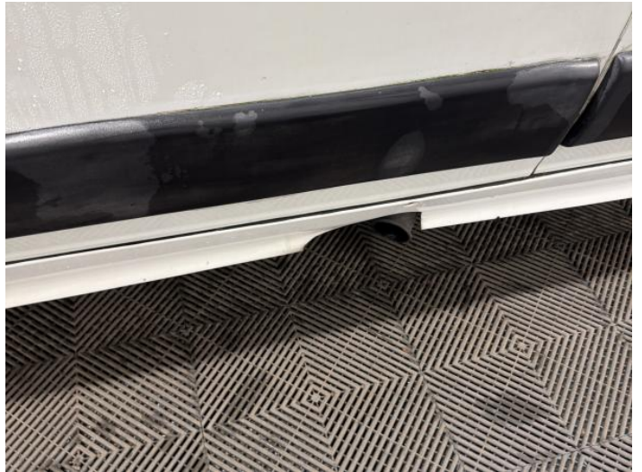
10: Sill Panel Trim os Scratched (Painted) Over 25mm Thru Paint
