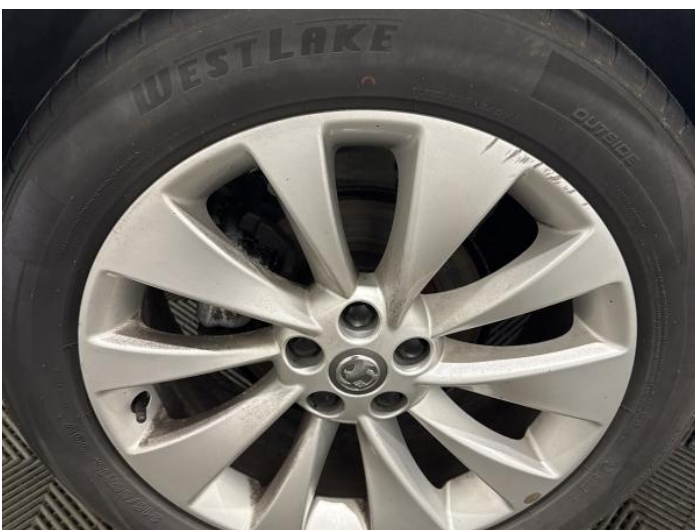
13: Wheel osr Scratched Over 50mm
