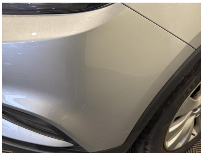
2: Bumper Front Scratched 25 to 100mm Thru Paint
