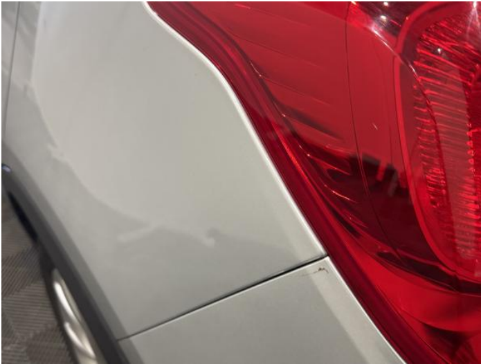
9: Qtr Panel nsr Dented Between 10mm + 30mm
