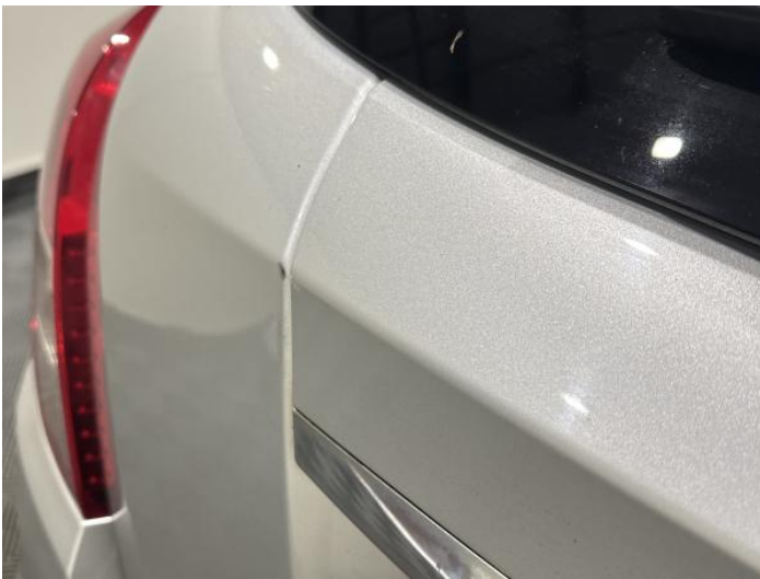
11: Tailgate Scratched UpTo 25mm Thru Paint
