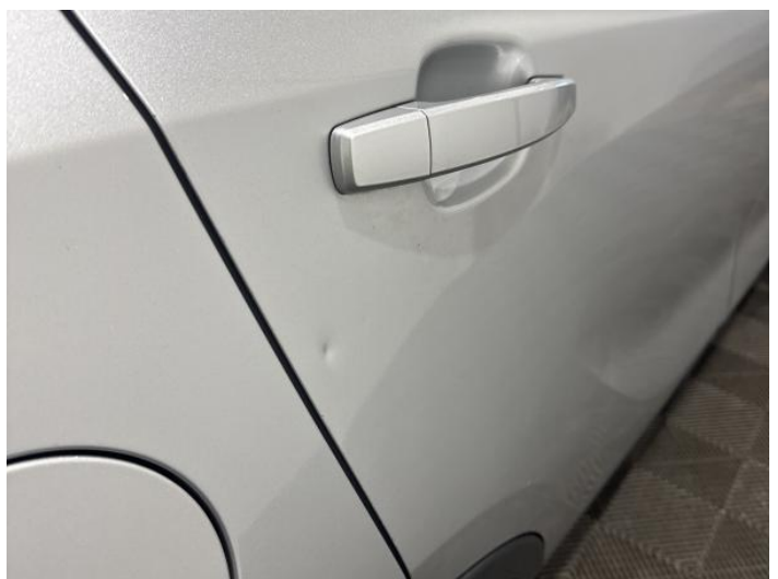
14: Door osr Dented Between 10mm + 30mm
