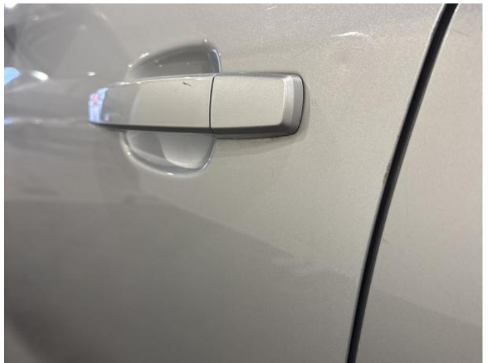
6: Door nsf Dented Between 10mm + 30mm
