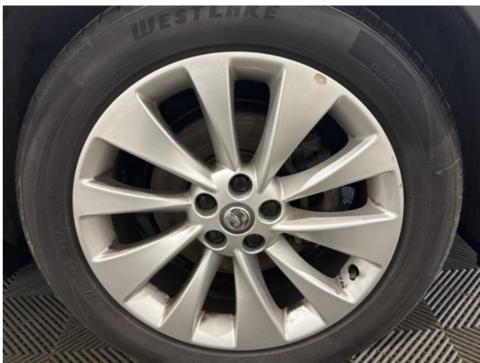
17: Wheel osf Scratched Up To 50mm
