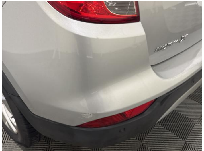
10: Bumper Rear Scratched 25 to 100mm Thru Paint
