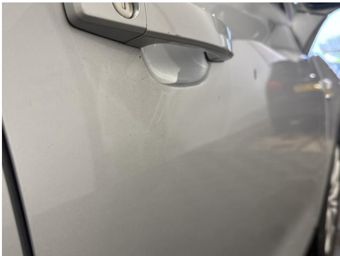
15: Door osf Dented Over 30mm
