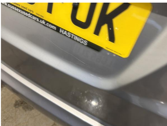
13: Boot Lid Scratched Over 25mm Thru Paint
