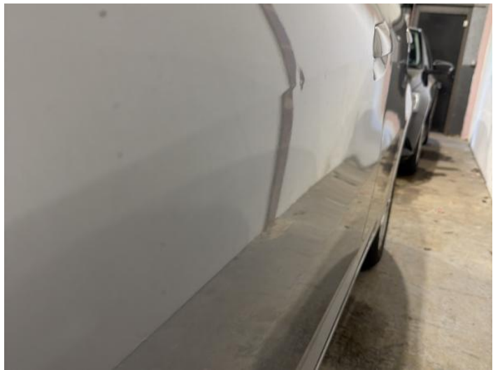
6: Door nsr Dented 2 Or Less UpTo 10mm
