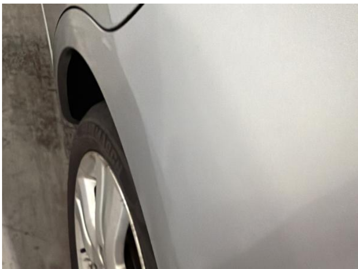
9: Qtr Panel nsr Dented Over 2 UpTo 10mm
