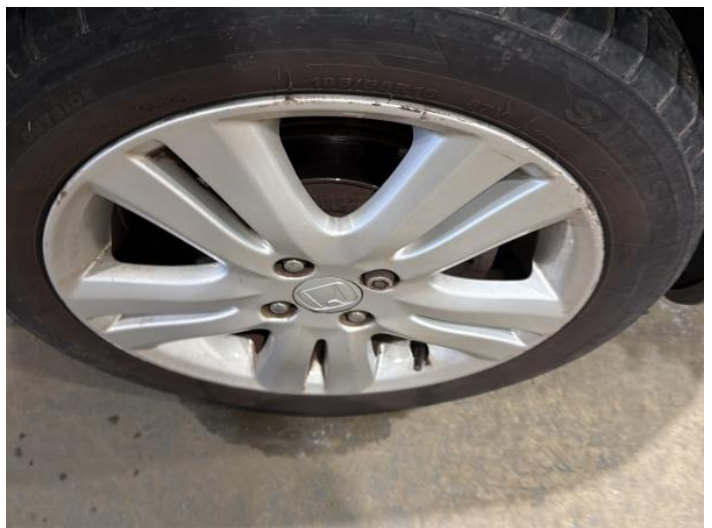
20: Wheel osf Scratched Over 50mm
