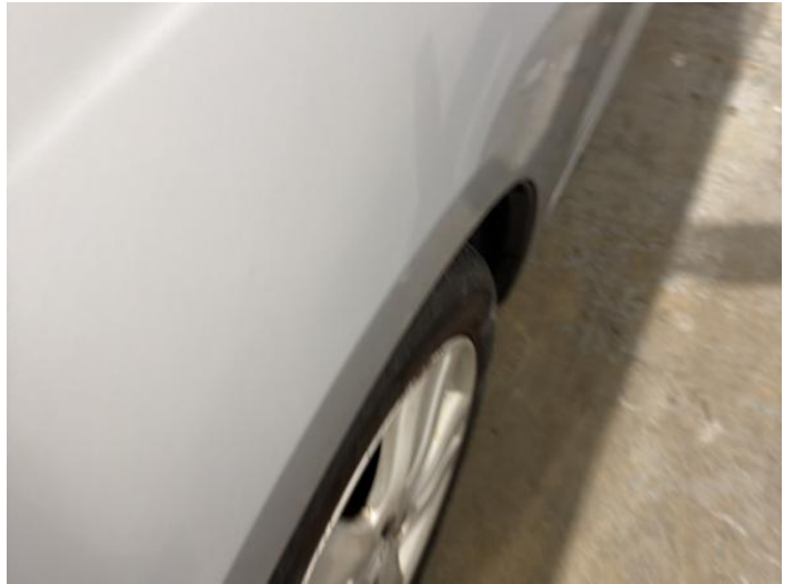
4: Wing nsf Dented Over 2 UpTo 10mm
