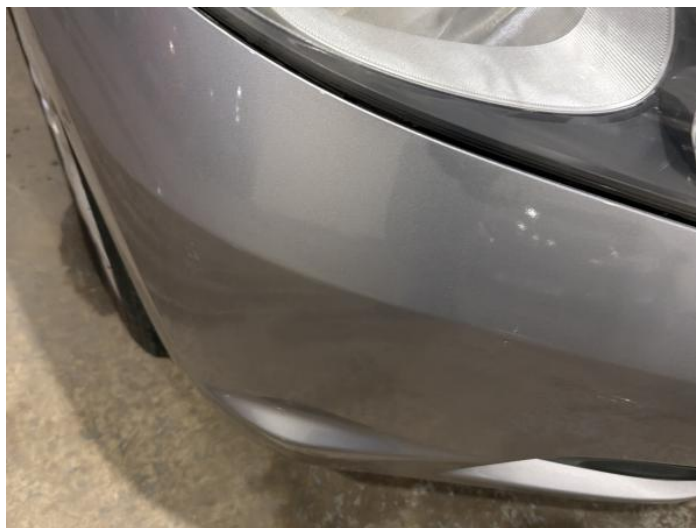
2: Bumper Front Scratched 25 to 100mm Thru Paint
