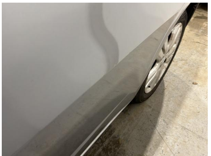
8: Door nsr Dented Over 30mm
