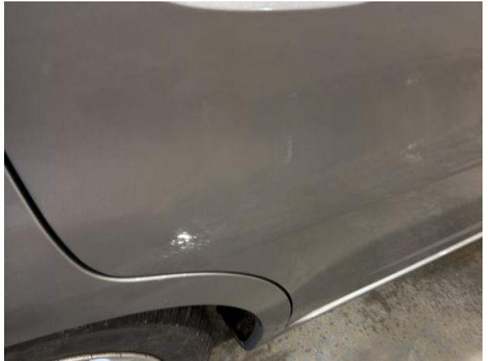
16: Door osr Poor Previous Repair Poor Paint
