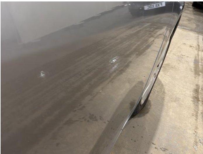
17: Door osf Dented Over 2 UpTo 10mm
