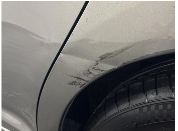
6: Qtr Panel nsr Dented Over 30mm
