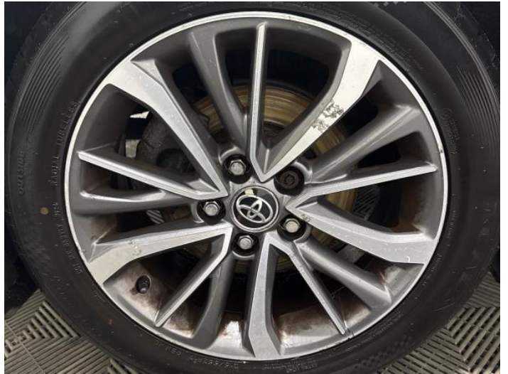
10: Wheel osr Corroded Light
