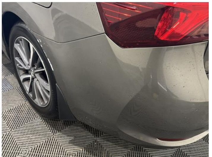
8: Bumper Rear Scratched Over 100mm Thru Paint
