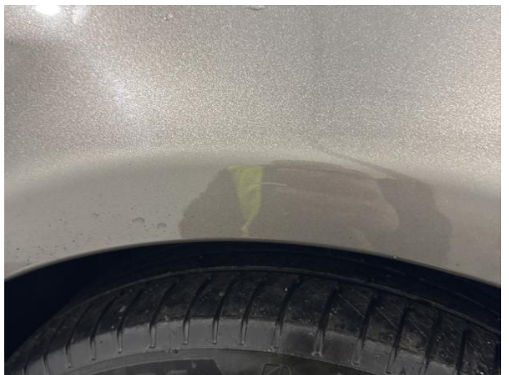
14: Wing osf Scratched UpTo 25mm Thru Paint
