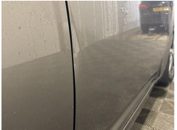
12: Door osf Dented Over 30mm
