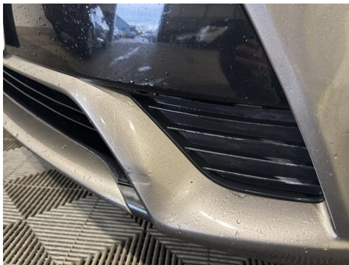
2: Bumper Front Dented With Paint Damage
