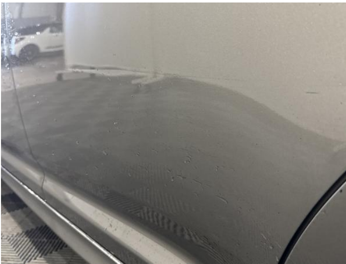
5: Door nsr Dented Over 30mm
