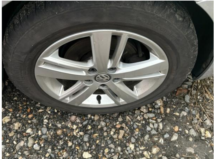
10: Wheel osf Scratched Over 50mm
