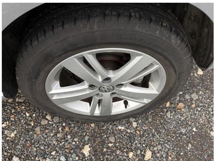
20: Wheel nsr Scratched Up To 50mm
