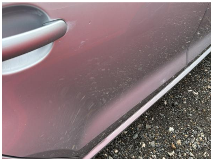
6: Door osr Scratched Over 25mm Thru Paint
