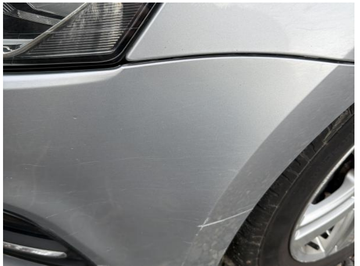
12: Bumper Front Scratched Over 100mm Thru Paint
