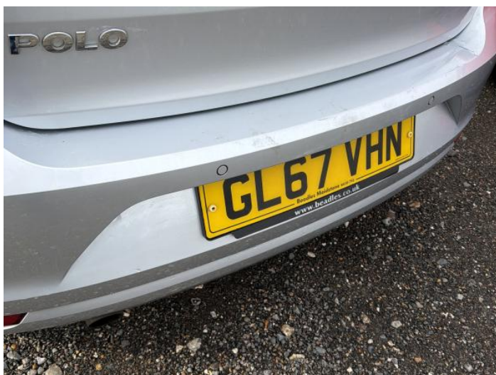
1: Bumper Rear Scratched Over 100mm Thru Paint
