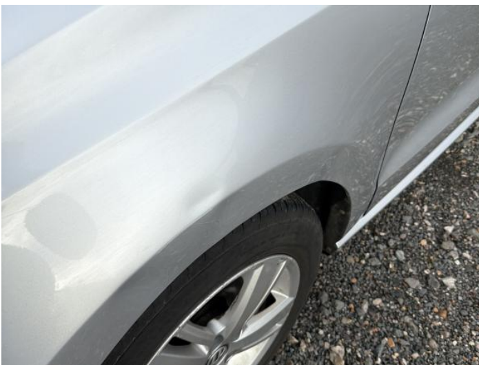
13: Wing nsf Dented With Paint Damage
