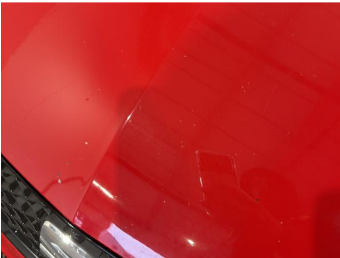
1: Bonnet Chipped Multiple Chips
