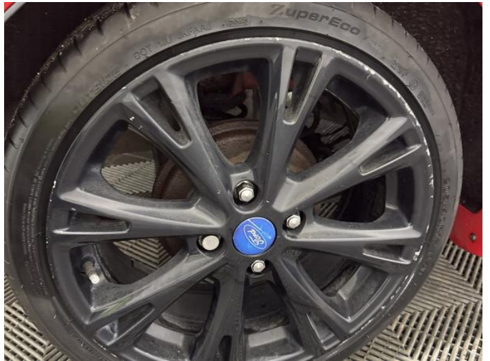
12: Wheel osr Scratched Over 50mm
