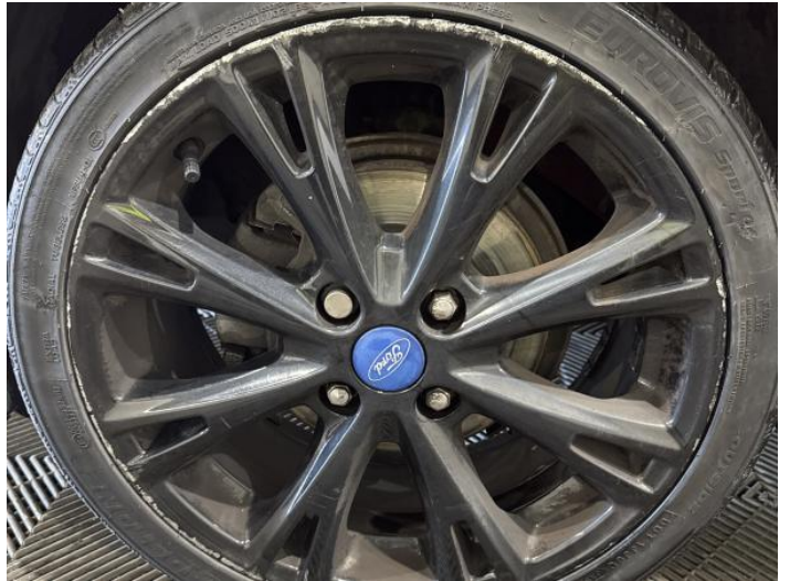
4: Wheel nsf Scratched Over 50mm
