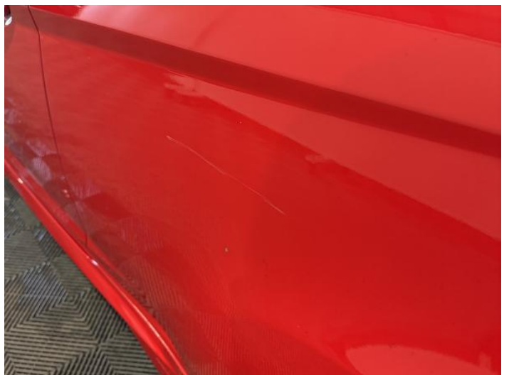
8: Qtr Panel nsr Dented Between 10mm + 30mm
