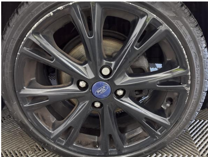
15: Wheel of Scratched Over 50mm
