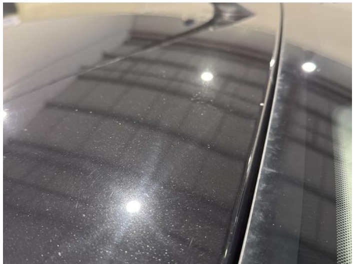
18: Roof Chipped Edge Chip
