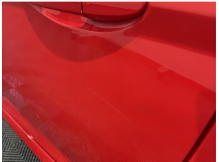
6: Door nsf Scratched Over 25mm Thru Paint
