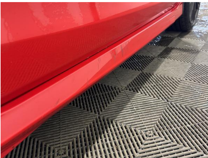
13: Sill Panel Trim os Scratched (Painted) Over 25mm Thru Paint
