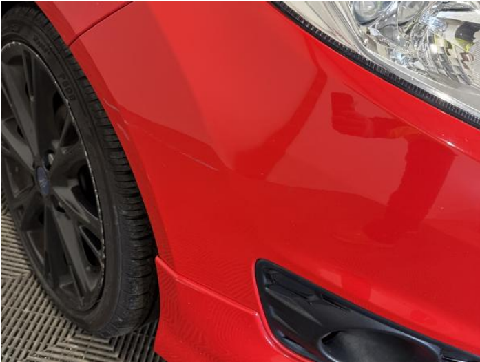
3: Bumper Front Scratched 25 to 100mm Thru Paint
