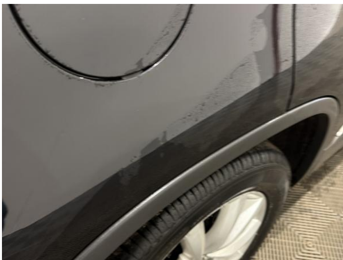
17: Qtr Panel osr Scratched Over 25mm Thru Paint
