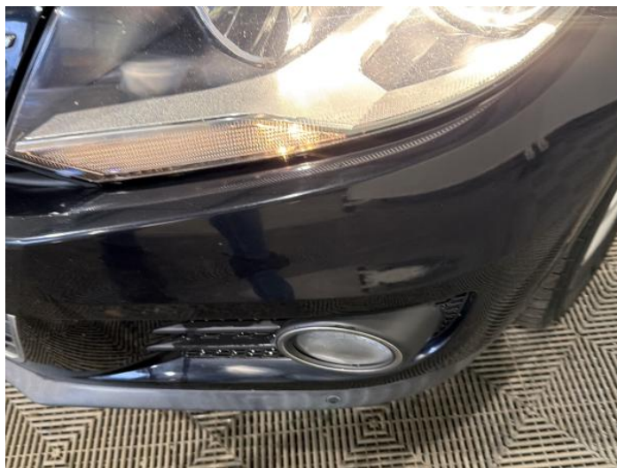
2: Bumper Front Chipped Multiple Chips
