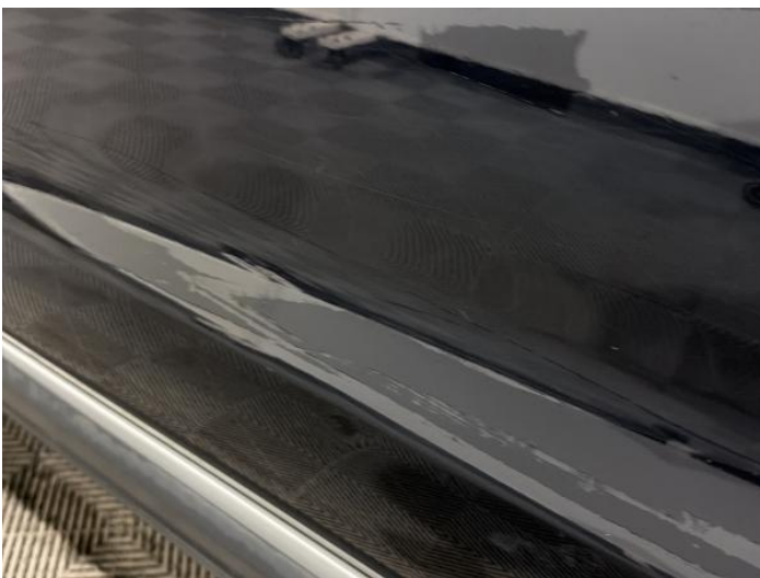
7: Door nsf Chipped Multiple Chips
