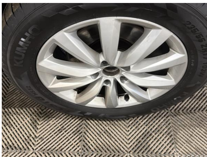
24: Wheel osf Scratched Up To 50mm
