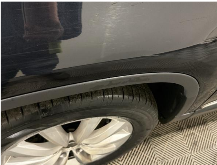
5: Wing nsf Dented Over 2 UpTo 10mm
