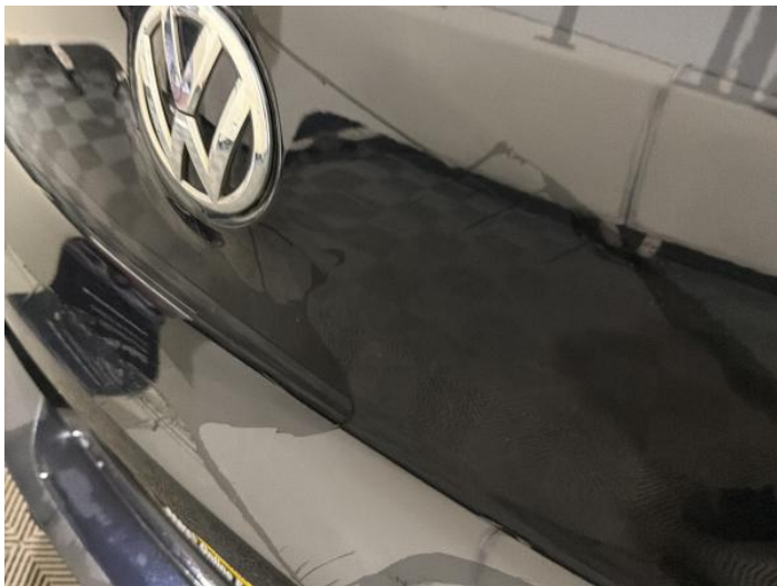
15: Boot Lid Dented Over 2 UpTo 10mm
