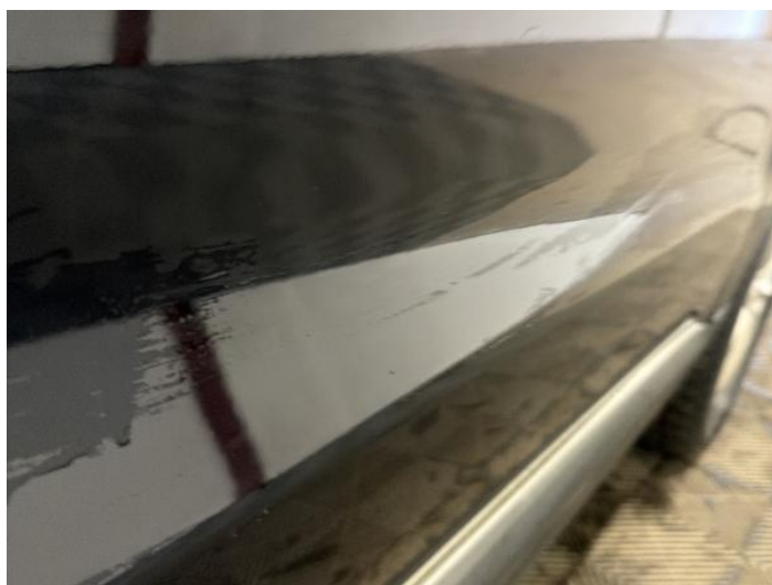
20: Door osf Dented Over 2 UpTo 10mm
