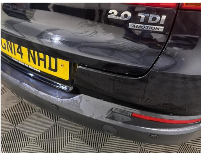
13: Bumper Rear Scratched 25 to 100mm Thru Paint
