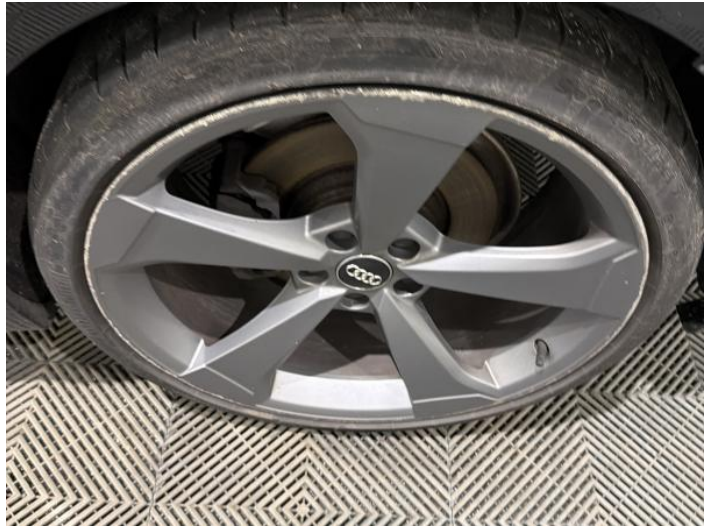
10: Wheel nsr Scratched Over 50mm
