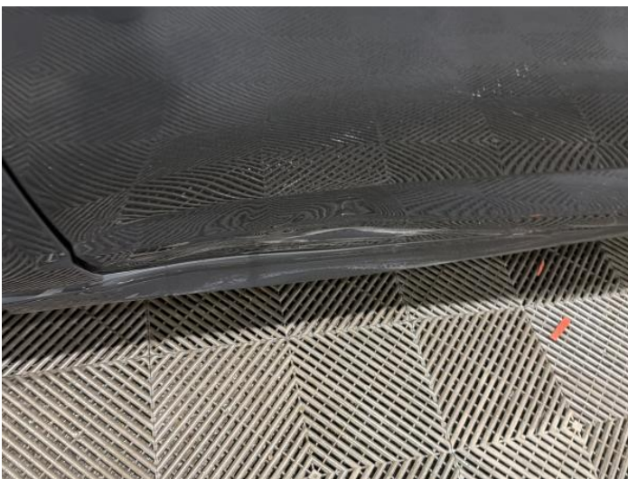
7: Sill ns Dented With Paint Damage
