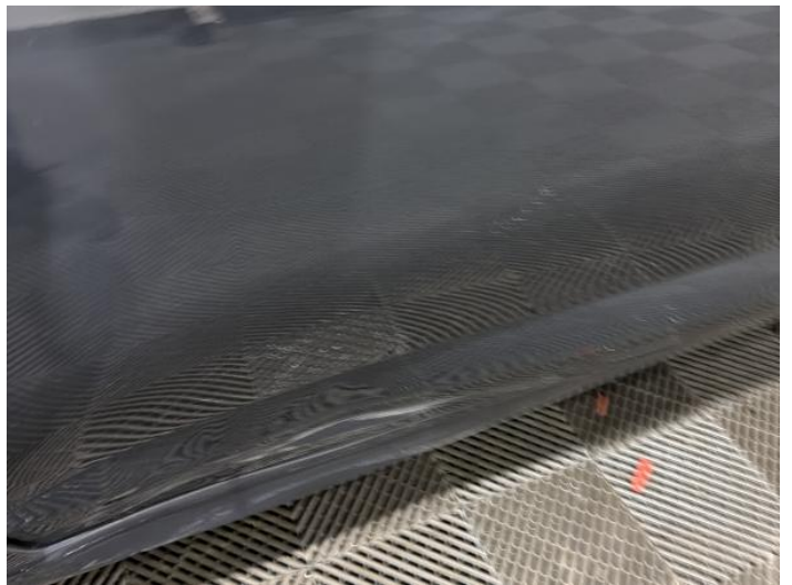
6: Door nsf Dented With Paint Damage
