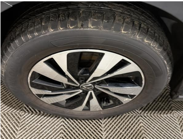
5: Wheel nsf Scratched Up To 50mm
