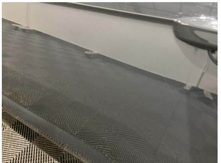
8: Door nsr Scratched Up To 25mm Thru Paint
