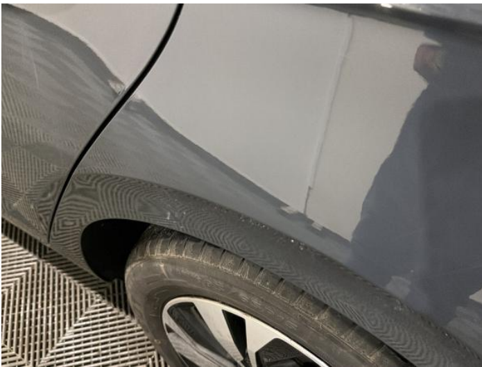
11: Qtr Panel nsr Dented Over 2 UpTo 10mm
