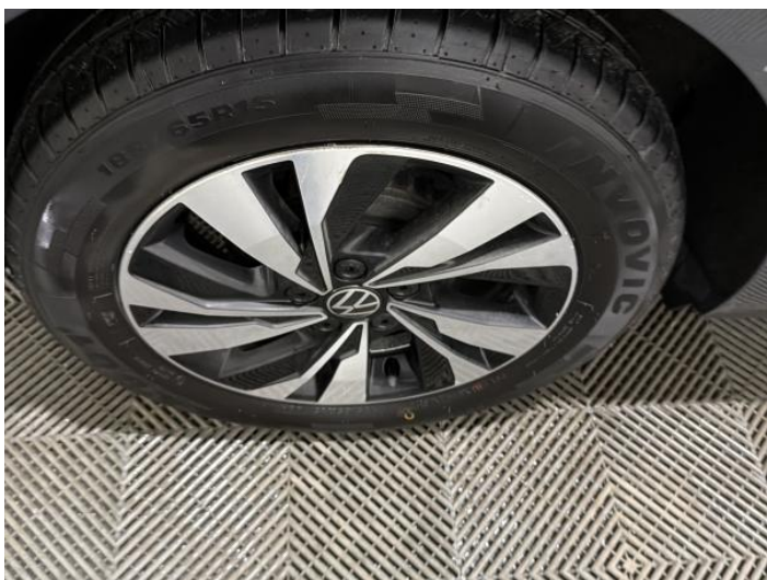
17: Wheel osr Scratched Up To 50mm
