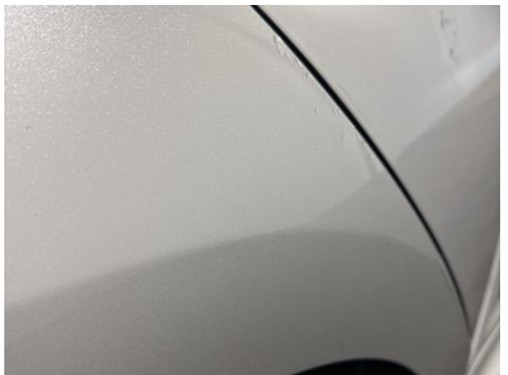
8: Qtr Panel osr Dented Between 10mm + 30mm
