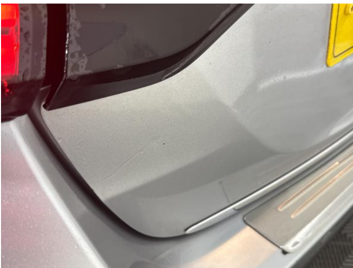
7: Tailgate Dented Between 10mm + 30mm
