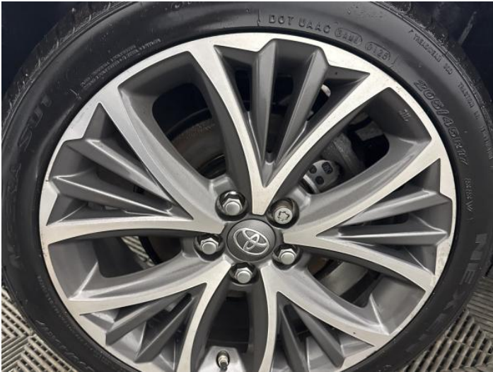
9: Wheel osr Scratched Up To 50mm
