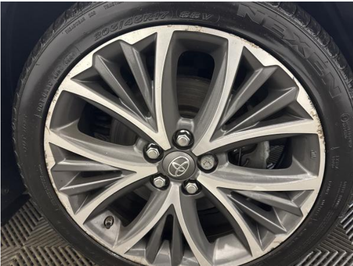
12: Wheel osf Scratched Over 50mm
