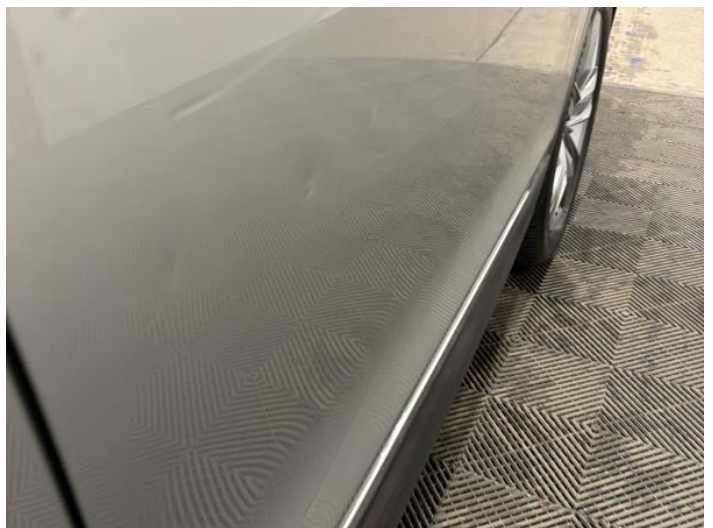
20: Door osf Dented Between 10mm + 30mm
