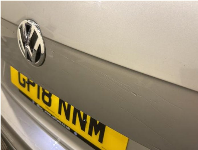
15: Boot Lid Dented 2 Or Less Up To 10mm
