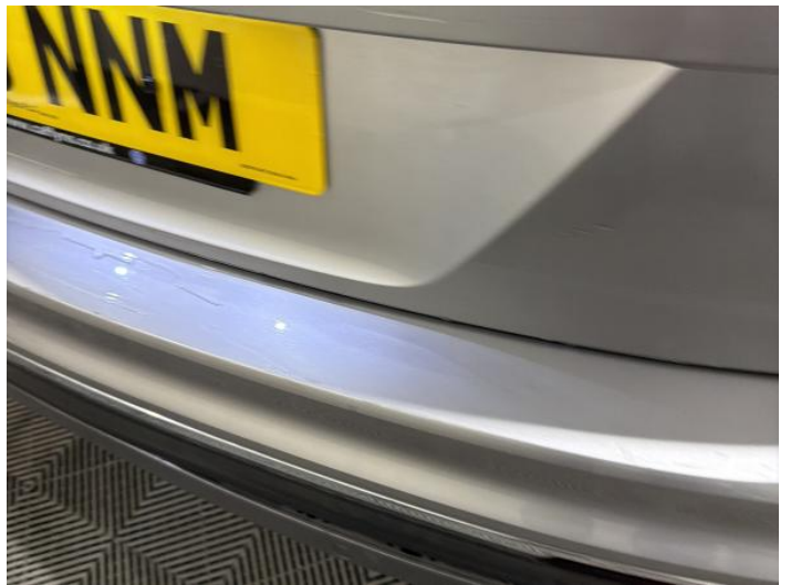
12: Bumper Rear Scratched 25 to 100mm Thru Paint
