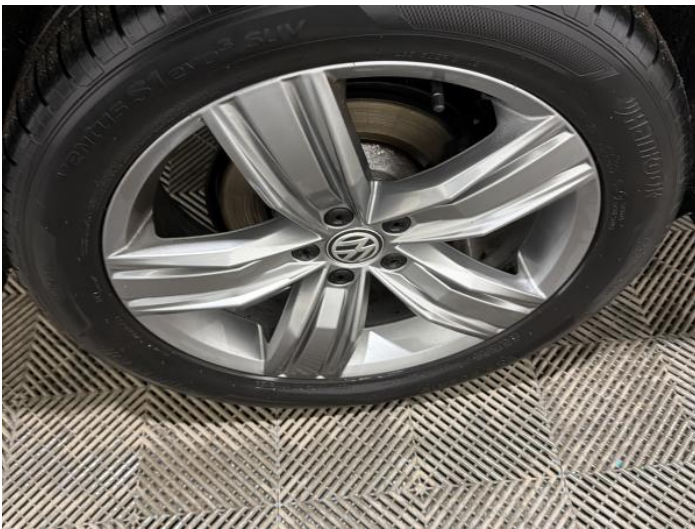
17: Wheel osr Scratched Up To 50mm
