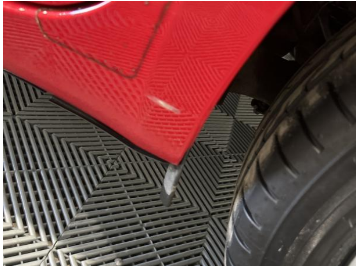
10: Sill ns Scratched UpTo 25mm Thru Paint
