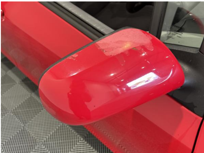
4: Door Mirror Assy osf Scratched (Painted) Over 25mm Thru Paint
