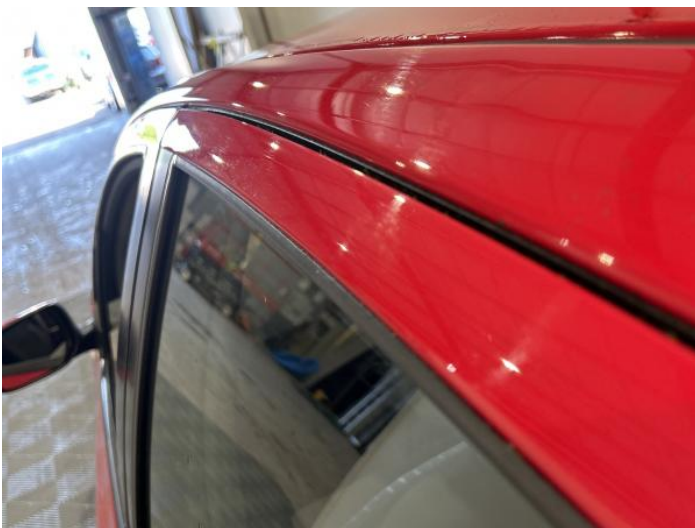
13: C Post ns Dented Between 10mm + 30mm
