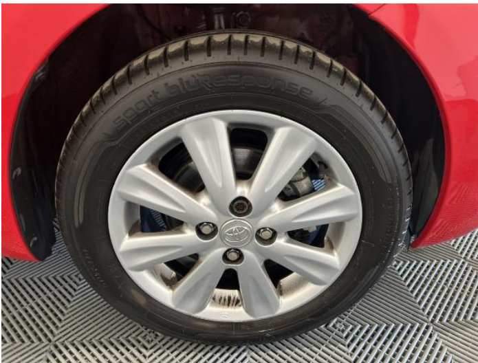
1: Wheel osf Scratched Over 50mm
