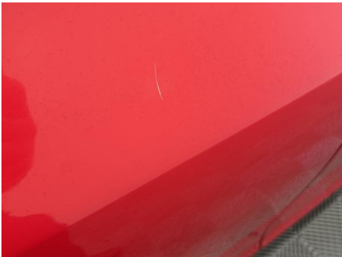
6: Door osr Scratched UpTo 25mm Thru Paint
