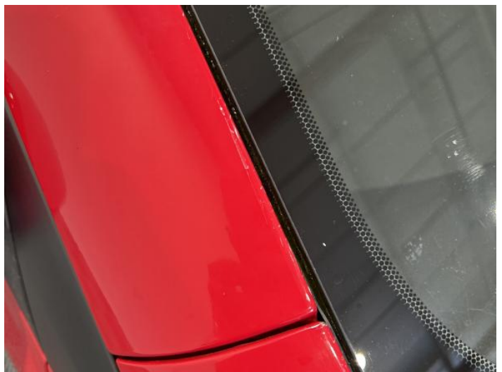
14: A Post os Poor Previous Repair Paint Flake
