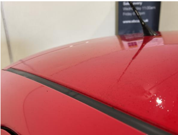
11: Roof Dented Over 2 UpTo 10mm
