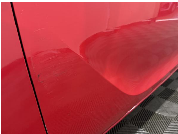
5: Door nsf Dented With Paint Damage
