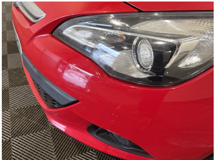
2: Bumper Front Scratched Over 100mm Thru Paint
