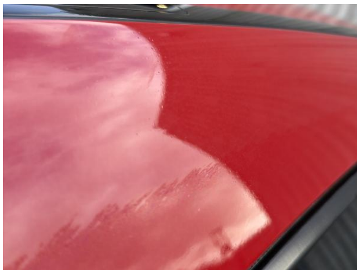
6: C Post os Poor Previous Repair Poor Paint
