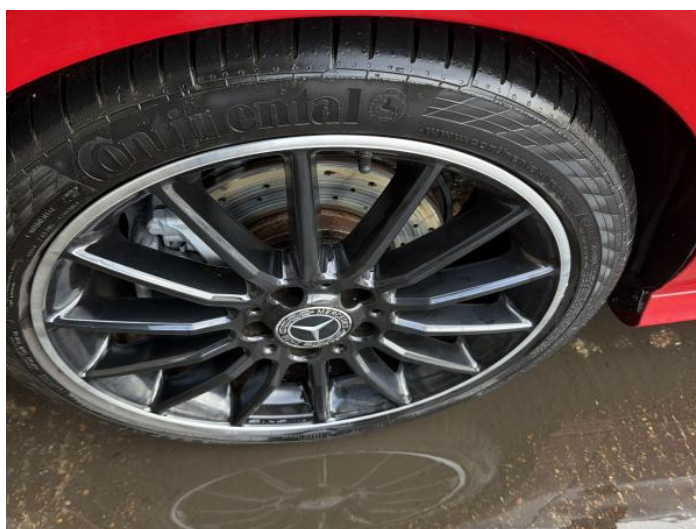
12: Wheel nsf Scratched Over 50mm
