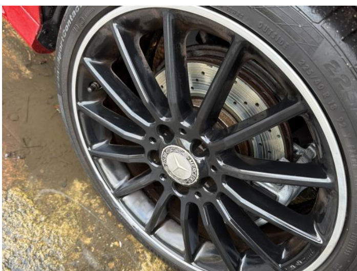
13: Wheel osf Scratched Over 50mm
