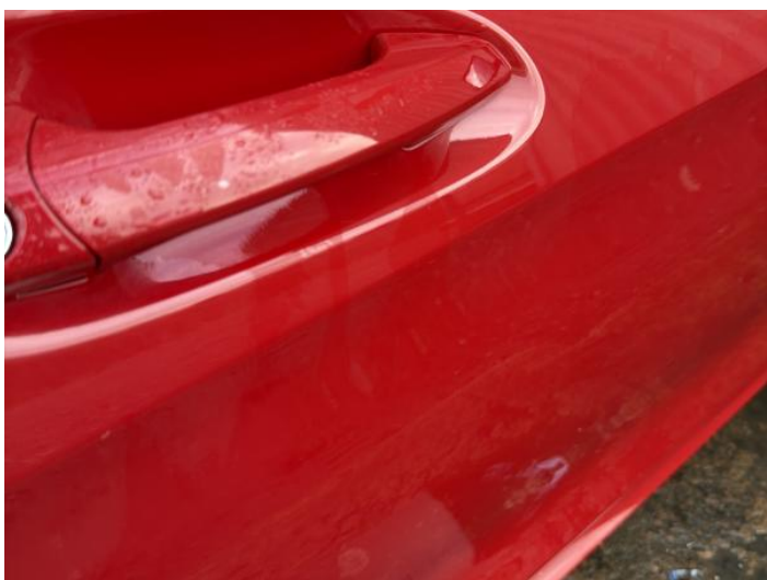
7: Door osf Poor Previous Repair Poor Paint
