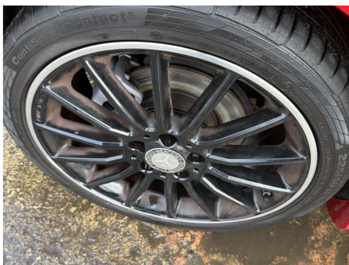
14: Wheel osr Scratched Over 50mm
