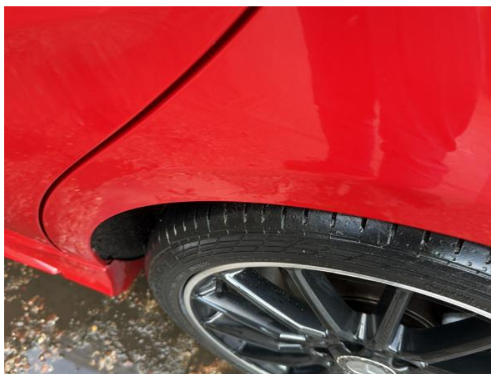
20: Qtr Panel nsr Dented Over 2 UpTo 10mm
