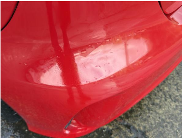
1: Bumper Rear Poor Previous Repair Poor Paint
