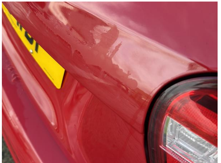
2: Boot Lid Dented With Paint Damage
