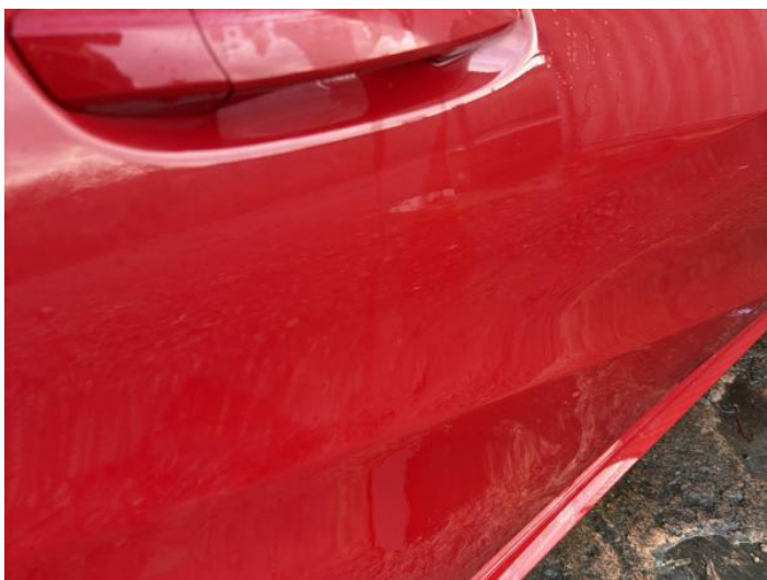
5: Door osr Poor Previous Repair Poor Paint
