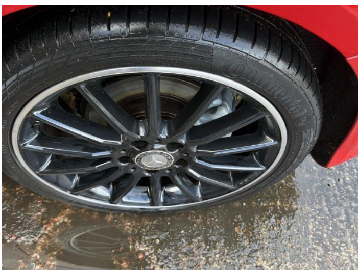
19: Wheel nsr Scratched Up To 50mm
