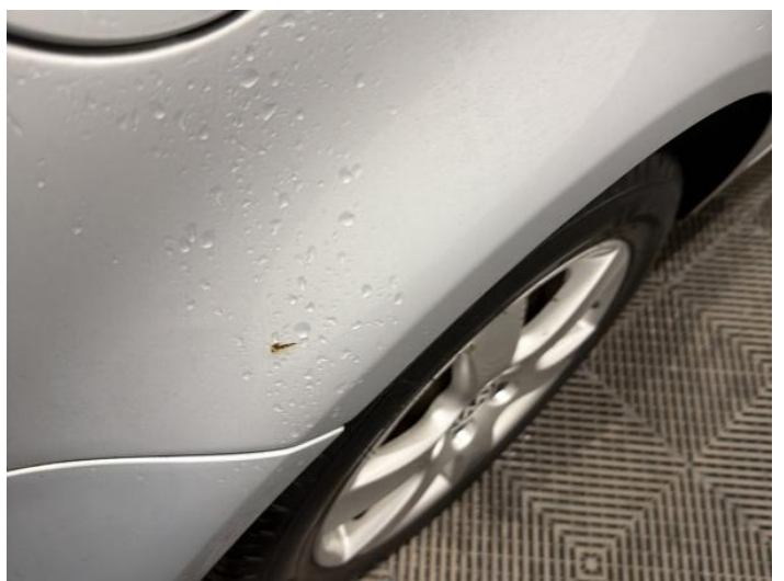
14: Qtr Panel osr Rusted UpTo 5mm
