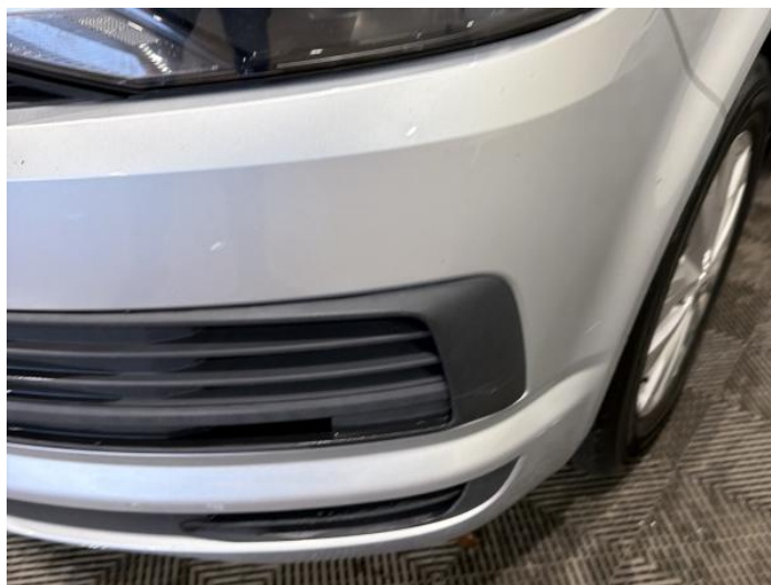
2: Bumper Front Scratched Over 100mm Thru Paint
