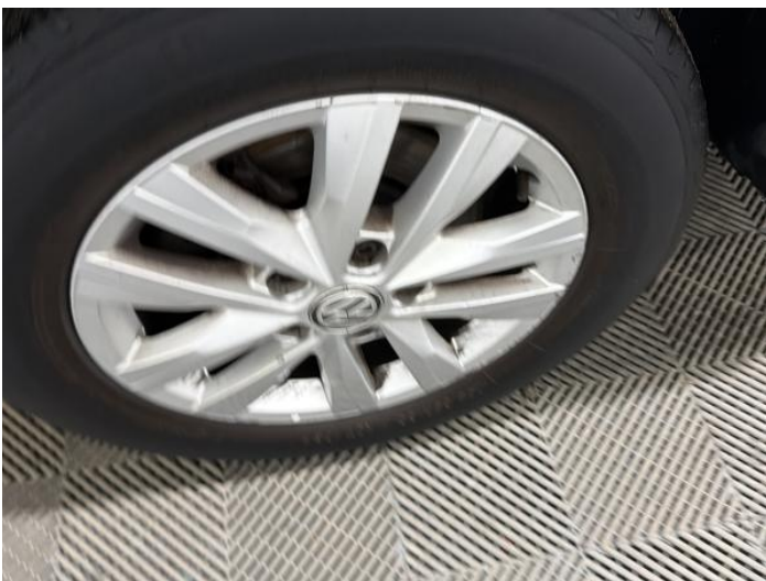
13: Wheel osr Scratched Over 50mm
