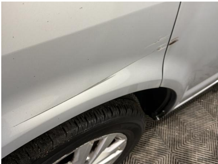
3: Wing nsf Dented With Paint Damage
