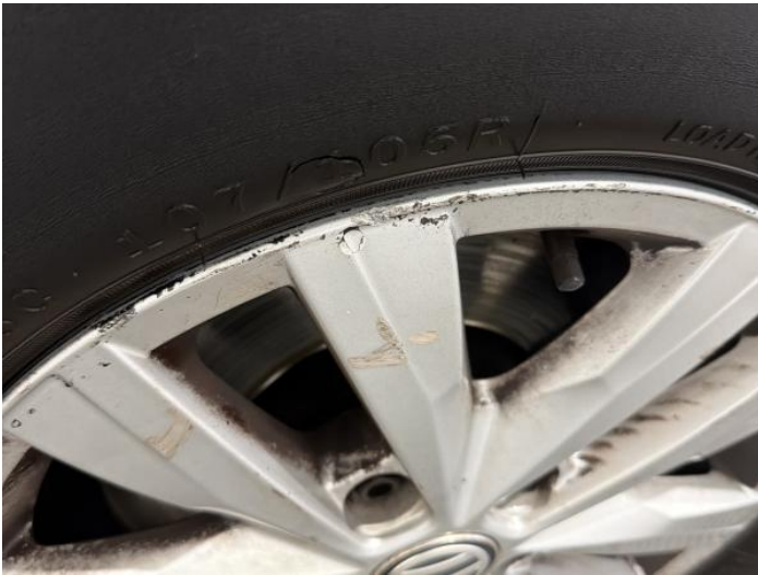
17: Tyre osf Damaged Replace
