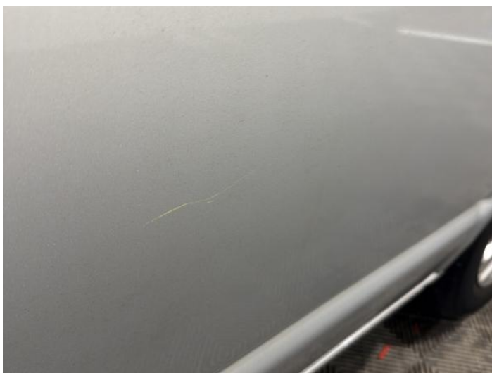
7: Door nsr Scratched Over 25mm Thru Paint
