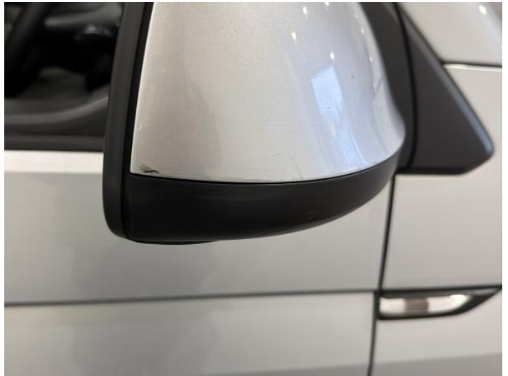
18: Door Mirror Assy osf Scratched (Painted) UpTo 25mm Thru Paint
