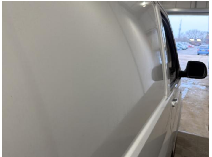
12: Qtr Panel osr Dented Over 30mm
