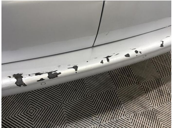
10: Bumper Rear Poor Previous Repair Rippled UpTo 30%
