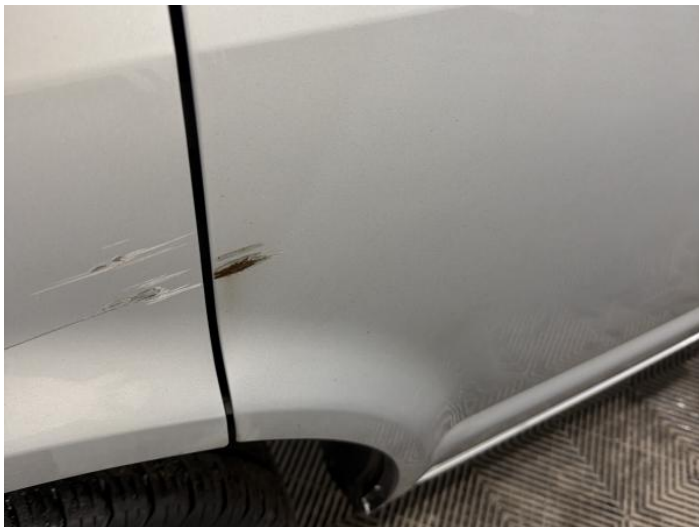
5: Door nsf Dented With Paint Damage
