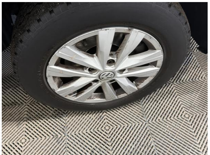
20: Wheel osf Scratched Over 50mm
