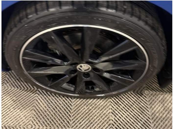
4: Wheel nsf Scratched Up To 50mm
