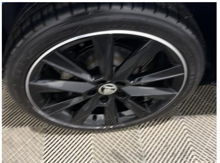
14: Wheel osr Scratched Up To 50mm
