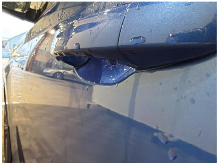
6: Door nsf Dented Over 2 UpTo 10mm
