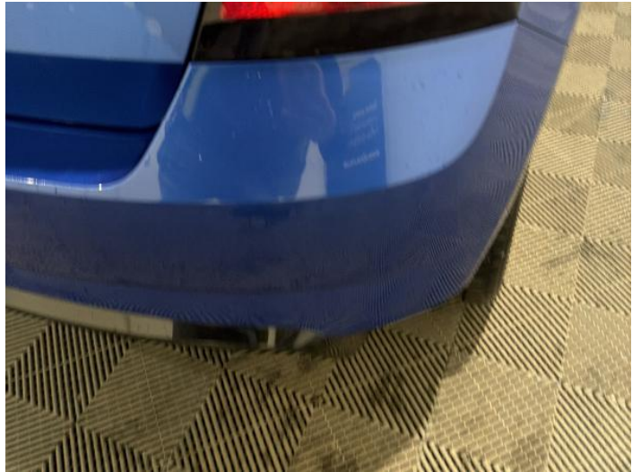
10: Bumper Rear Chipped Multiple Chips
