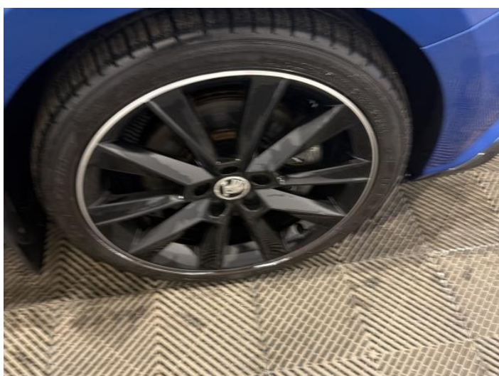
19: Wheel osf Scratched Up To 50mm
