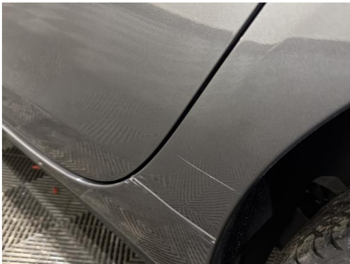
9: Qtr Panel nsr Dented With Paint Damage
