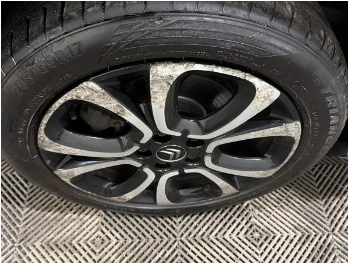
5: Wheel nsf Scratched Over 50mm
