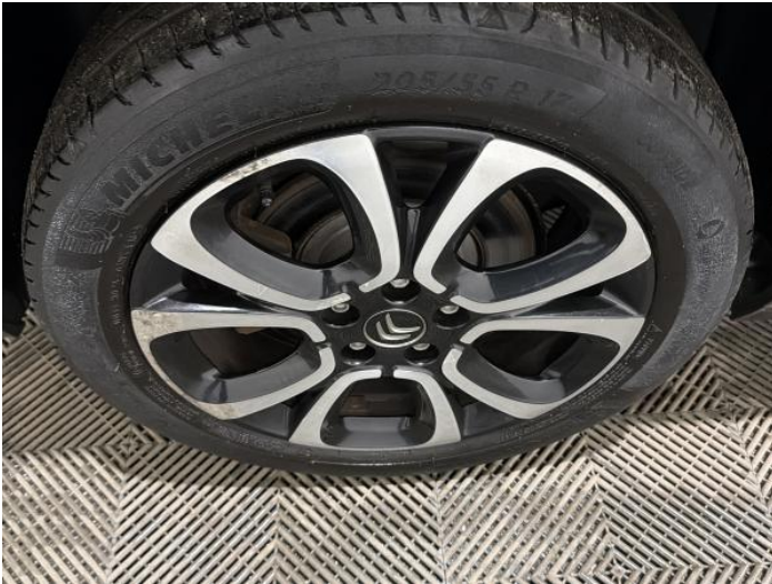
15: Wheel osr Scratched Over 50mm
