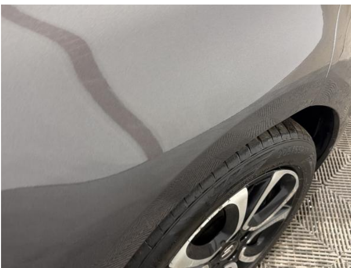
19: Wing osf Dented Between 10mm + 30mm
