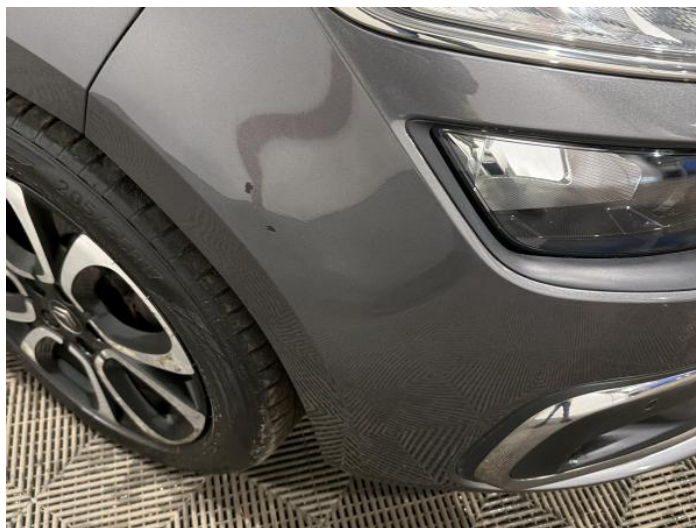
2: Bumper Front Scratched 25 to 100mm Thru Paint
