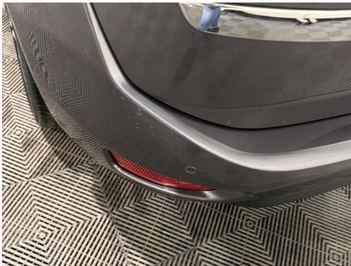
11: Bumper Rear Scratched 25 to 100mm Thru Paint
