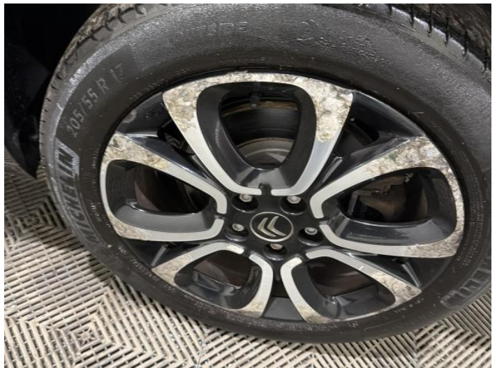
10: Wheel nsr Scratched Over 50mm
