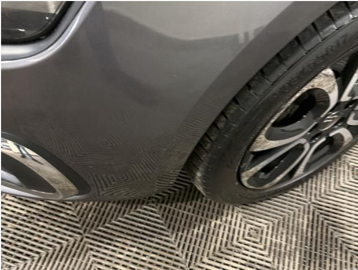
3: Bumper Front Scratched UpTo 25mm Thru Paint
