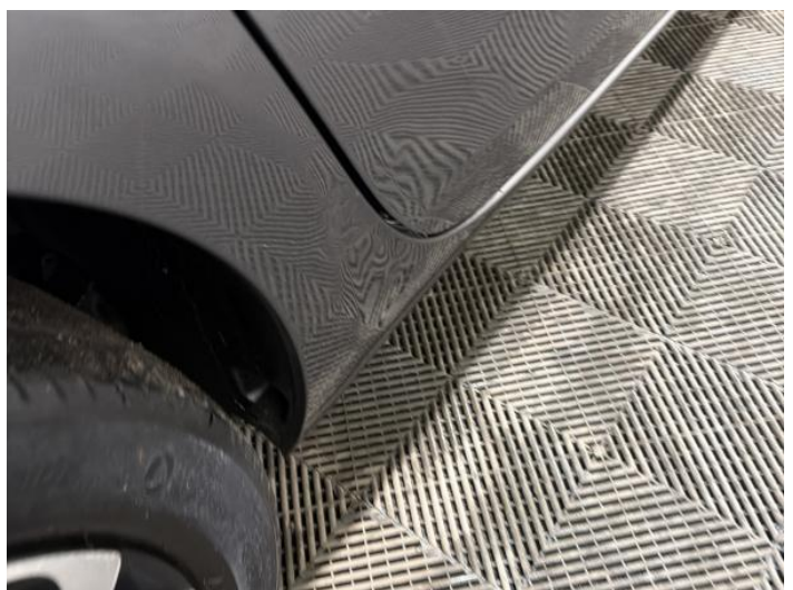
14: Qtr Panel osr Dented Over 30mm
