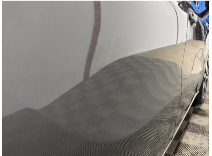
16: Door osr Poor Previous Repair Poor Paint
