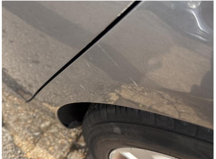
22: Qtr Panel nsr Dented Over 30mm
