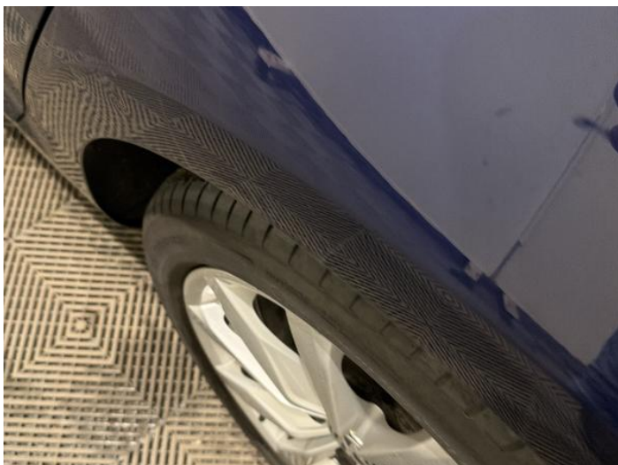
9: Qtr Panel nsr Dented With Paint Damage
