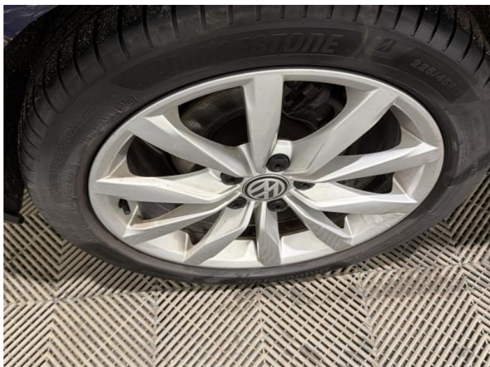
15: Wheel osr Scratched Up To 50mm
