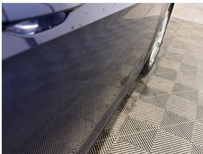
18: Door osf Poor Previous Repair Poor Paint
