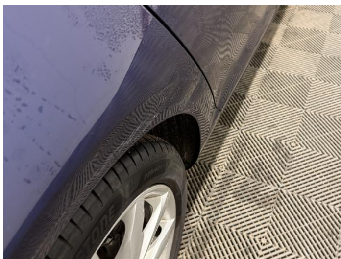
14: Qtr Panel osr Dented Over 30mm
