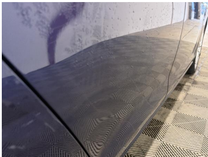
16: Door osr Scratched UpTo 25mm Thru Paint
