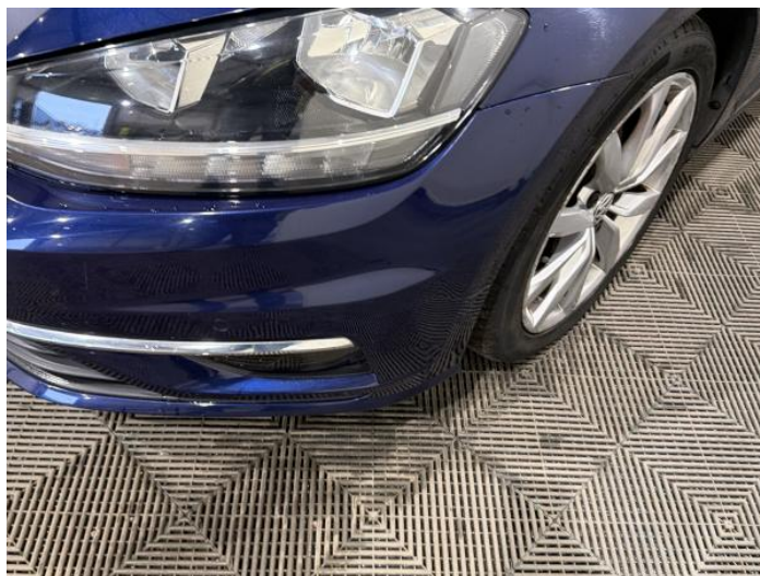
2: Bumper Front Scratched Over 100mm Thru Paint
