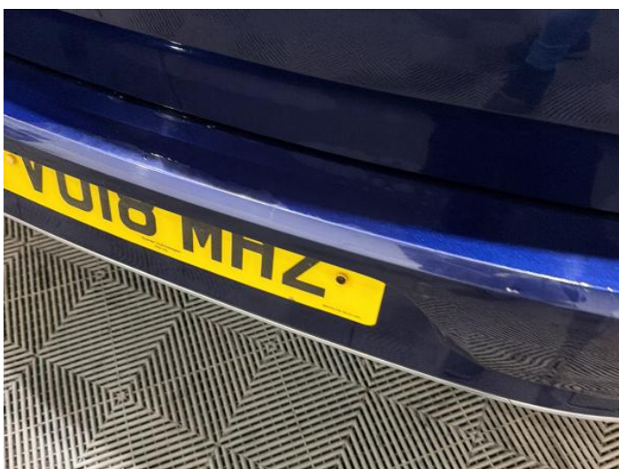
11: Bumper Rear Scratched 25 to 100mm Thru Paint
