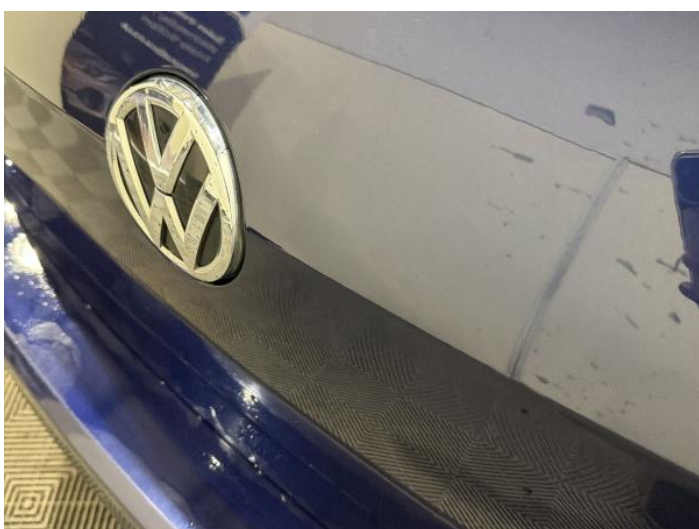
13: Boot Lid Dented Over 2 Up To 10mm
