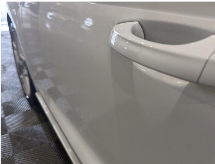
5: Door nsf Dented Over 2 UpTo 10mm
