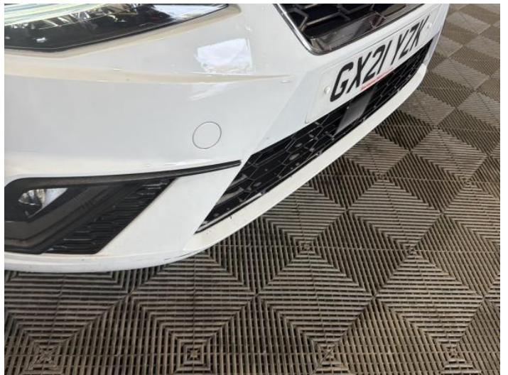
2: Bumper Front Scratched Over 100mm Thru Paint
