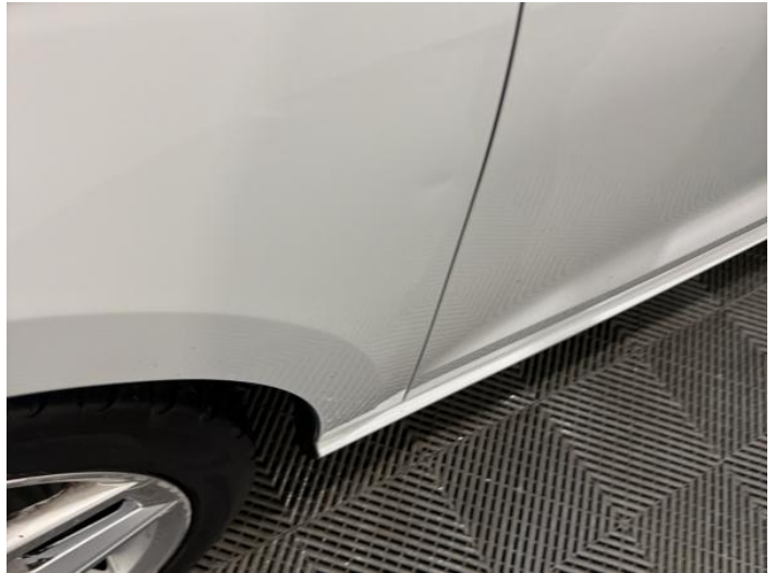
4: Wing nsf Dented Between 10mm + 30mm
