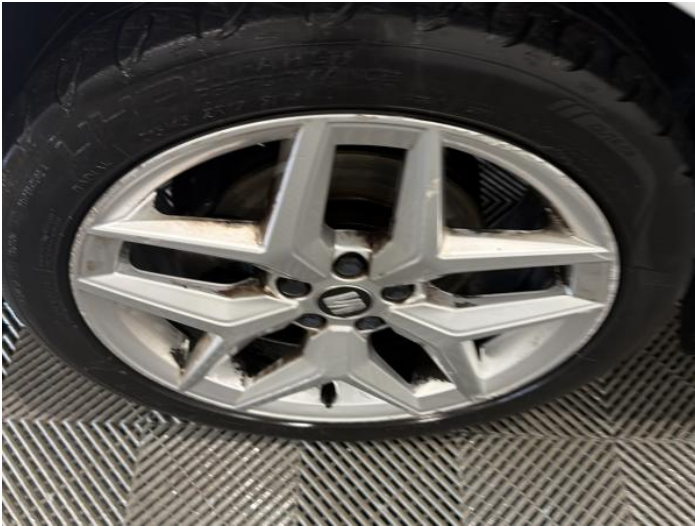
3: Wheel nsf Scratched Over 50mm
