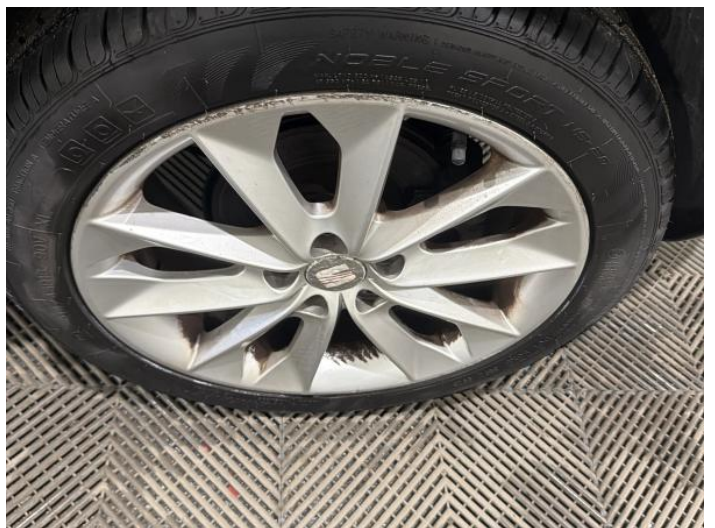
8: Wheel nsr Scratched Over 50mm
