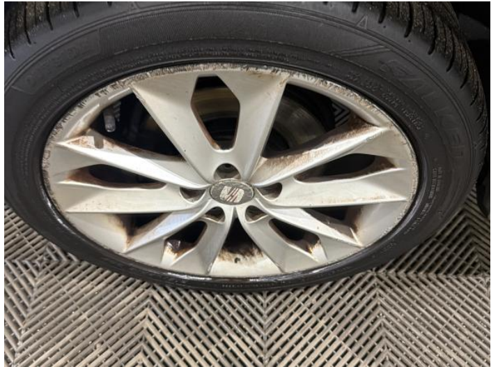
4: Wheel nsf Scratched Over 50mm
