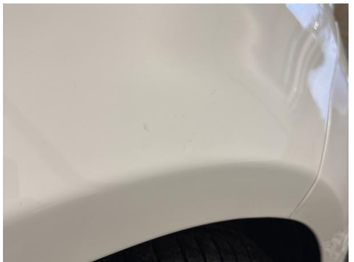
14: Wing osf Scratched UpTo 25mm Thru Paint
