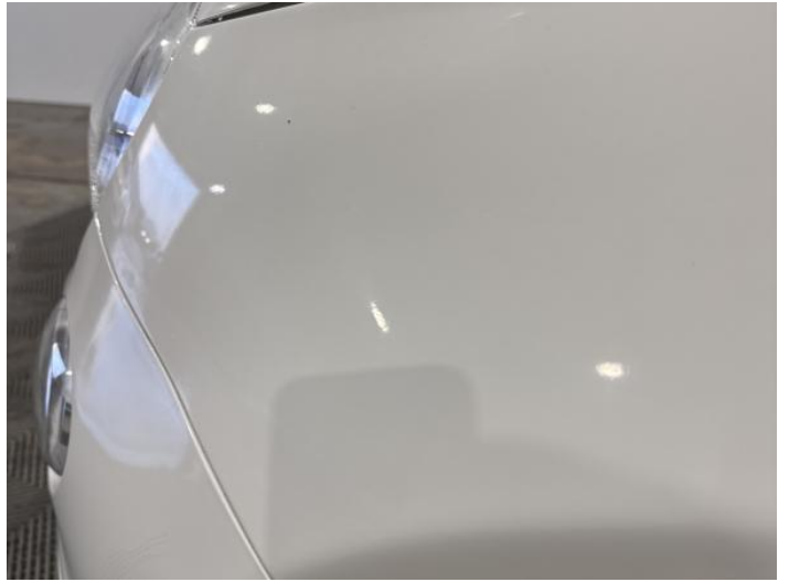
4: Wing nsf Poor Previous Repair Poor Paint
