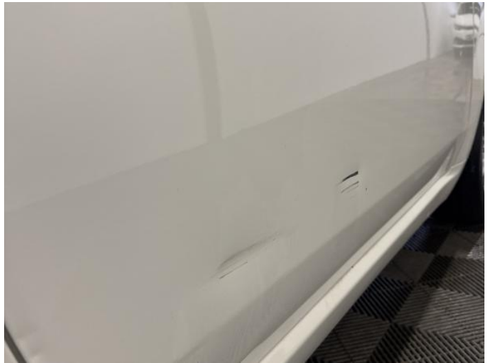
12: Door osf Dented With Paint Damage
