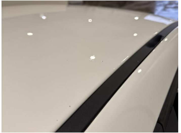
10: Roof Dented Over 30mm
