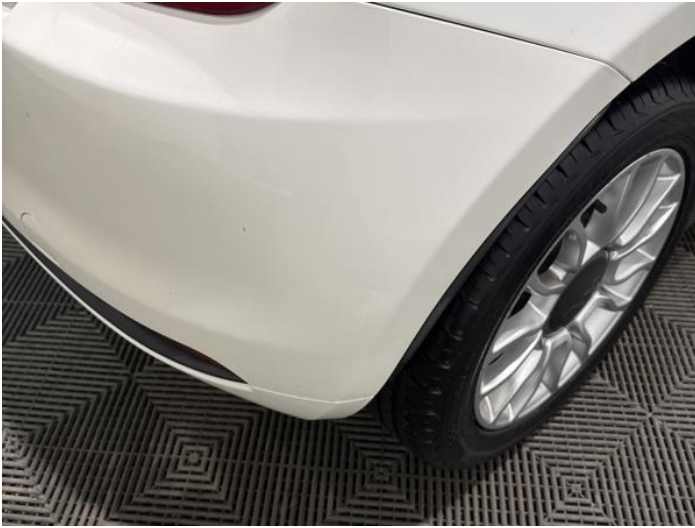
9: Bumper Rear Scratched Over 100mm Thru Paint
