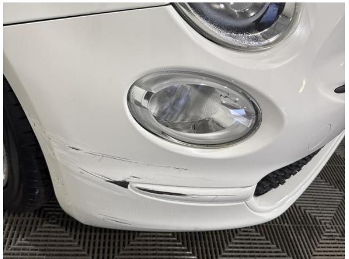
2: Bumper Front Scratched Over 100mm Thru Paint
