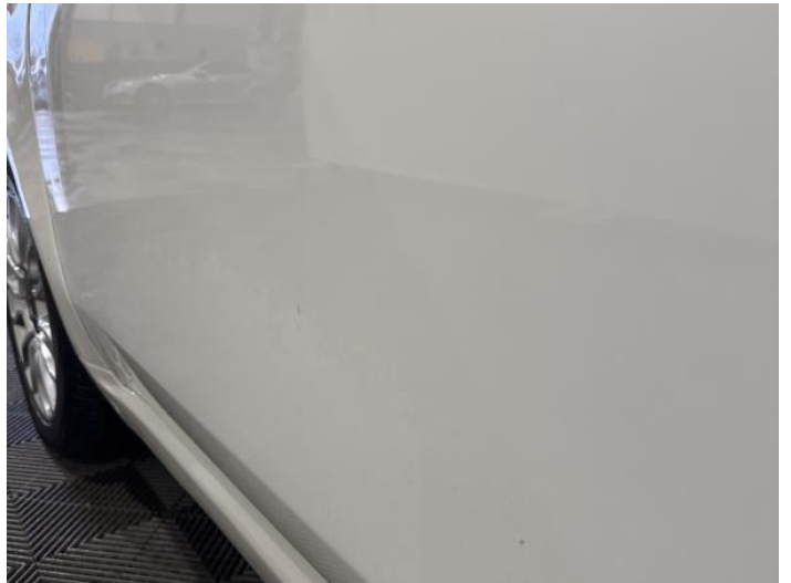
6: Door nsf Dented Over 30mm
