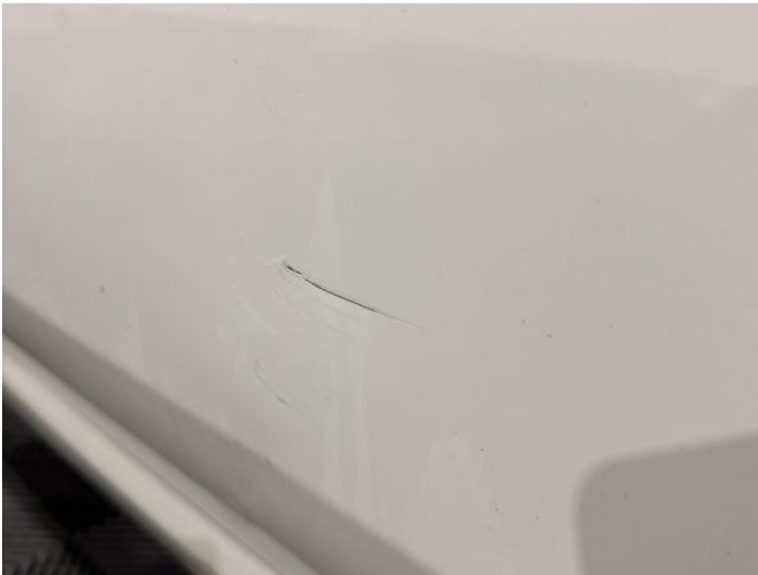
5: Door nsf Scratched Over 25mm Thru Paint
