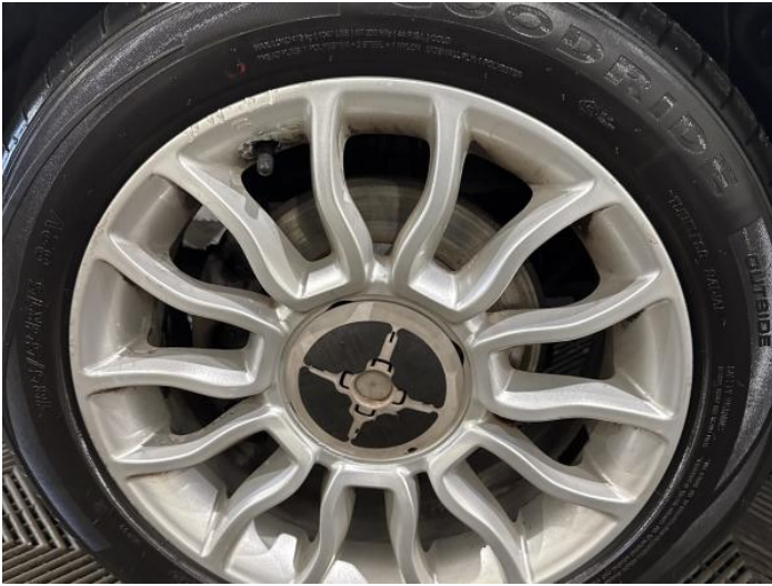
3: Wheel nsf Scratched Over 50mm
