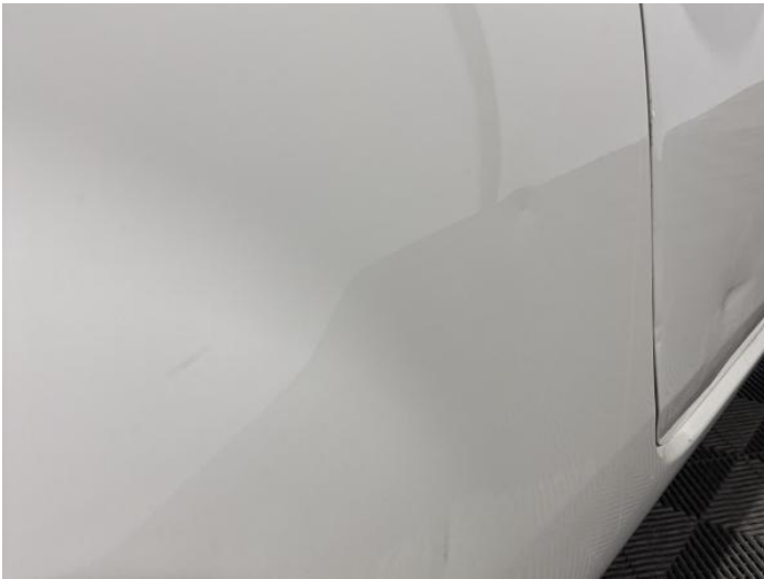
11: Qtr Panel osf Dented Between 10mm + 30mm
