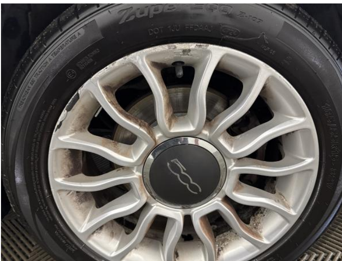
13: Wheel osf Scratched Over 50mm
