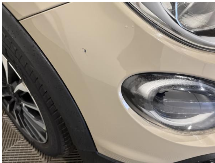
2: Bumper Front Scratched 25 to 100mm Thru Paint
