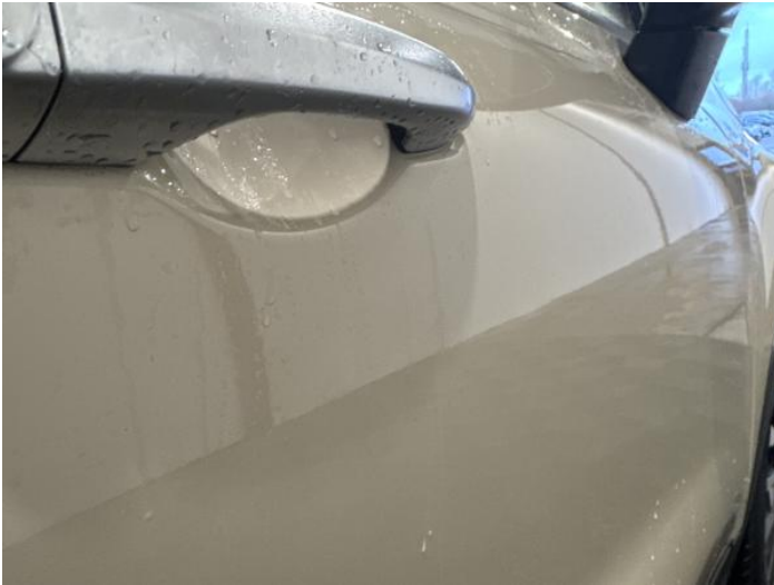
9: Door osf Dented Between 10mm + 30mm
