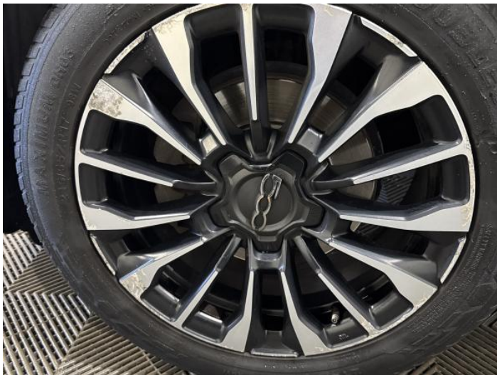
3: Wheel nsf Scratched Over 50mm
