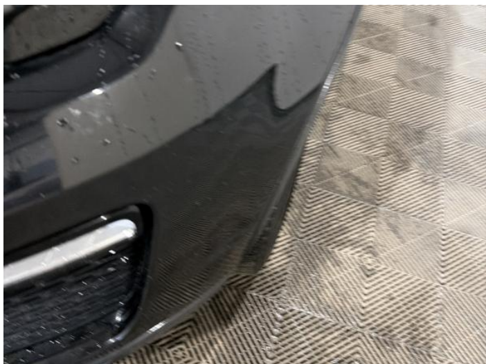
3: Bumper Front Chipped Multiple Chips
