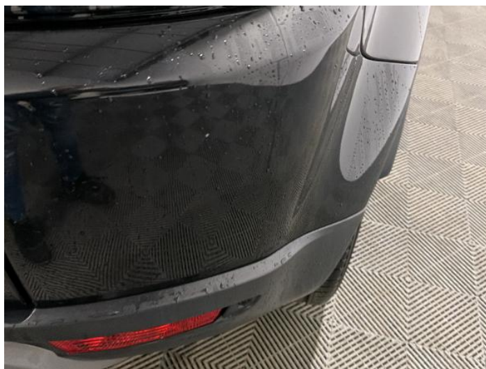
12: Bumper Rear Chipped Multiple Chips
