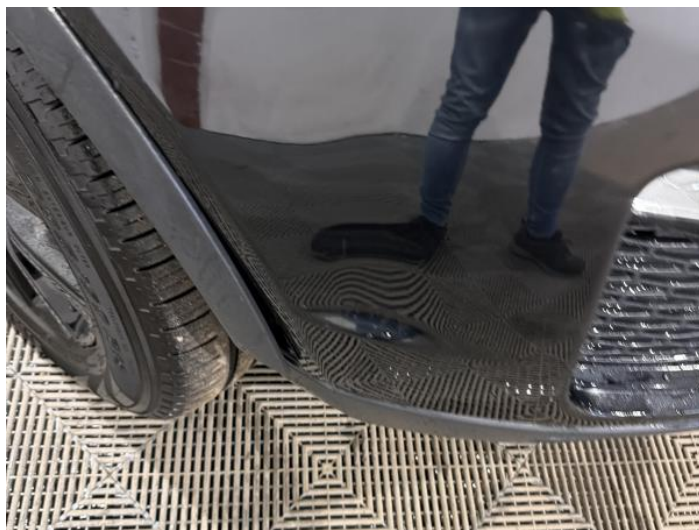
2: Wing Front Arch Extension os Broken Replace
