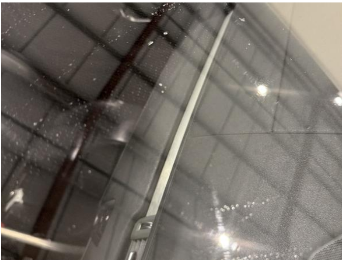
23: Screen Front Chipped UpTo 10mm
