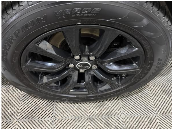
10: Wheel nsr Scratched Up To 50mm
