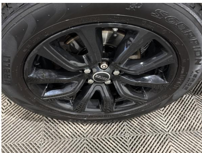
5: Wheel nsf Scratched Up To 50mm
