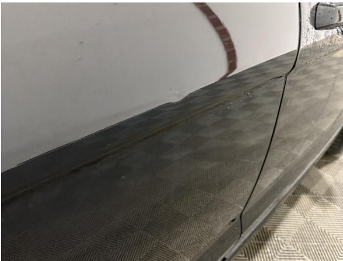
17: Door osr Dented Between 10mm + 30mm
