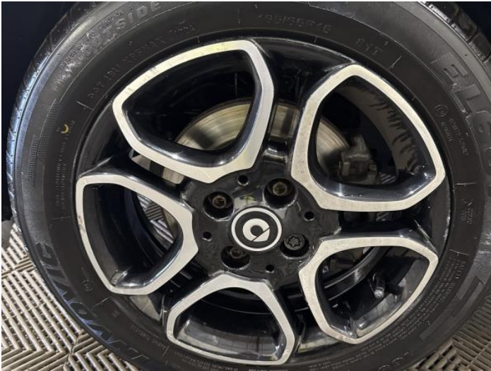
3: Wheel nsf Scratched Over 50mm
