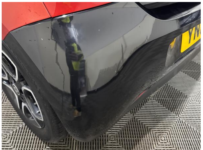
8: Bumper Rear Scratched 25 to 100mm Thru Paint
