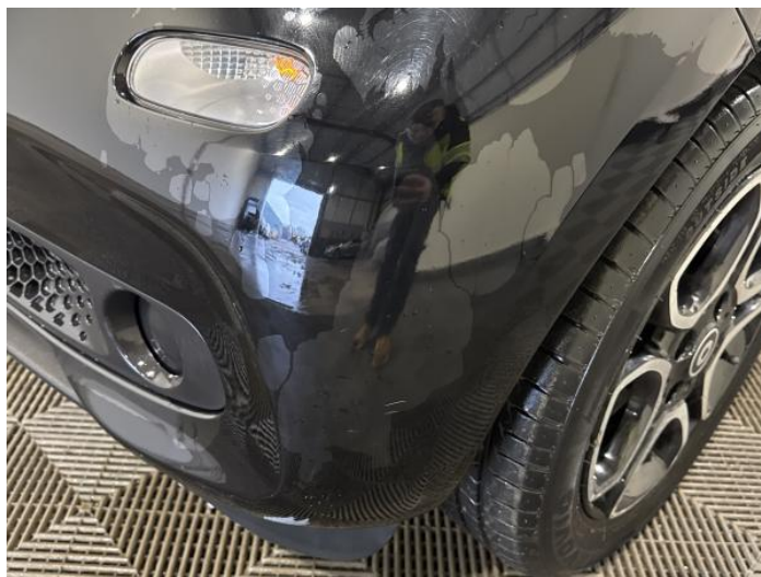
2: Bumper Front Scratched Over 100mm Thru Paint
