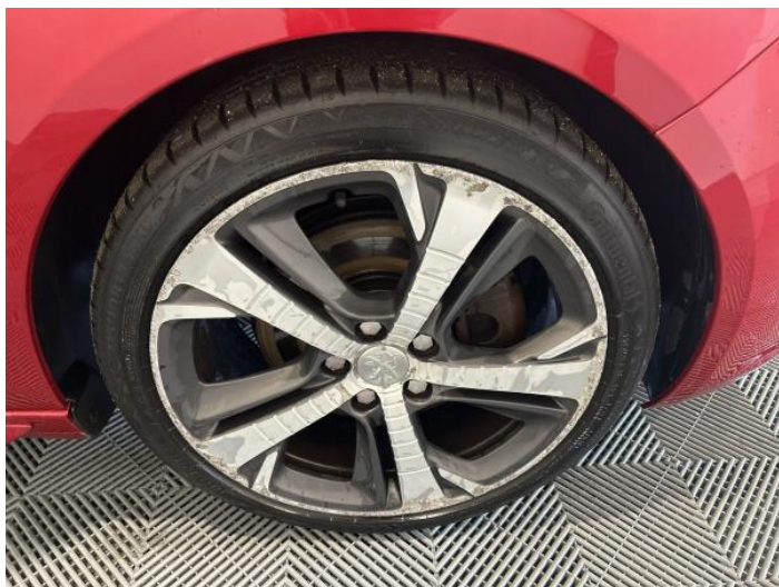
1: Wheel osf Scratched Over 50mm
