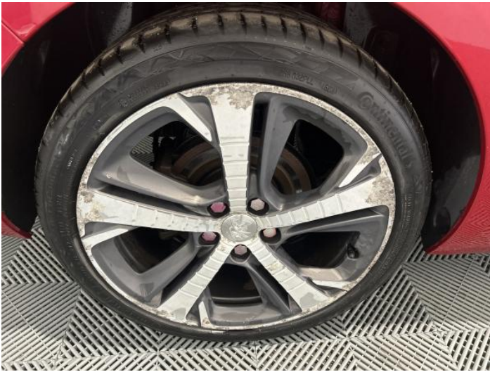
5: Wheel osr Scratched Over 50mm
