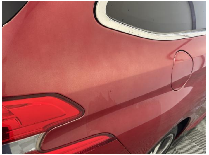
6: Qtr Panel osr Poor Previous Repair Poor Colour
