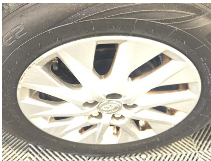
14: Wheel nsf Scratched Over 50mm
