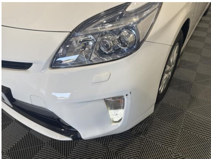
1: Bumper Front Scratched Over 100mm Thru Paint
