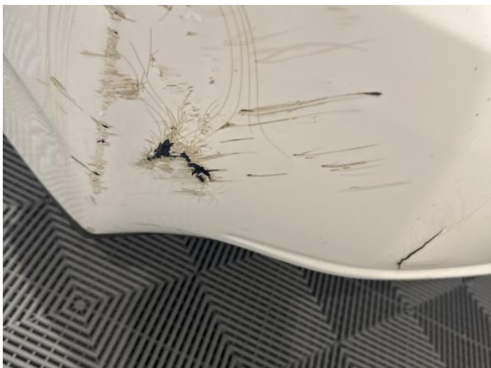
9: Bumper Rear Cracked UpTo 25mm
