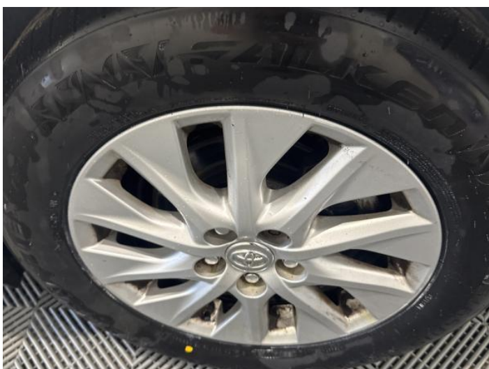
11: Wheel nsr Scratched Up To 50mm
