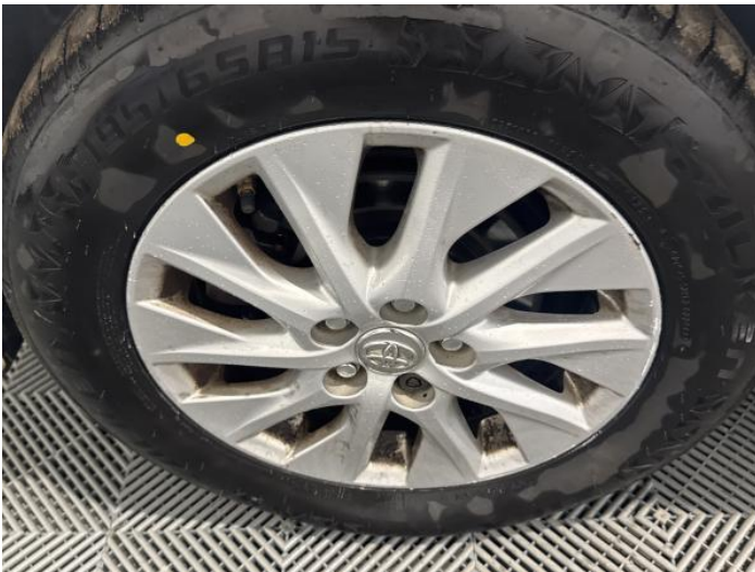
7: Wheel osr Scratched Over 50mm
