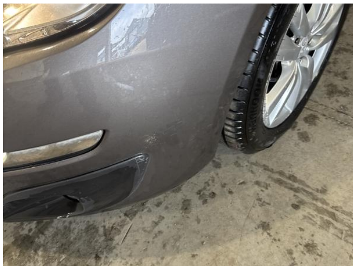
2: Bumper Front Scratched Over 100mm Thru Paint
