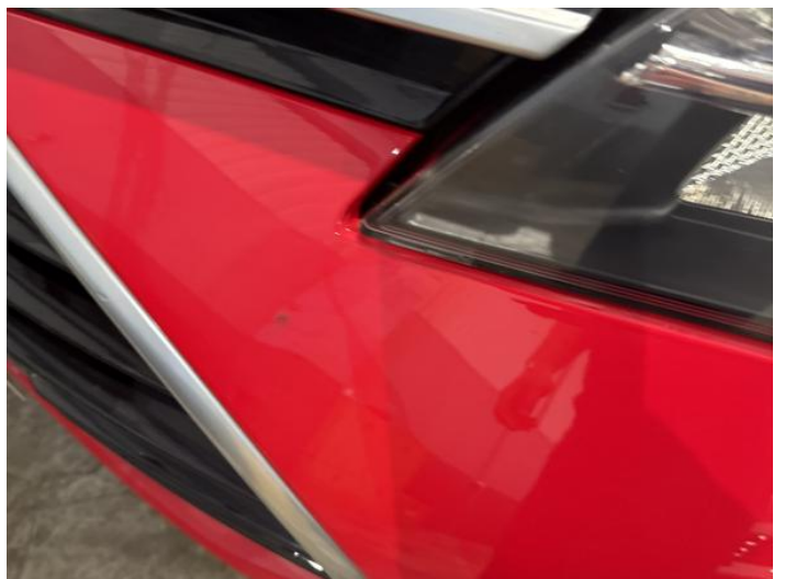
8: Bumper Front Chipped Multiple Chips
