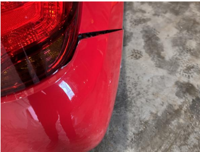
1: Bumper Rear Cracked Over 25mm
