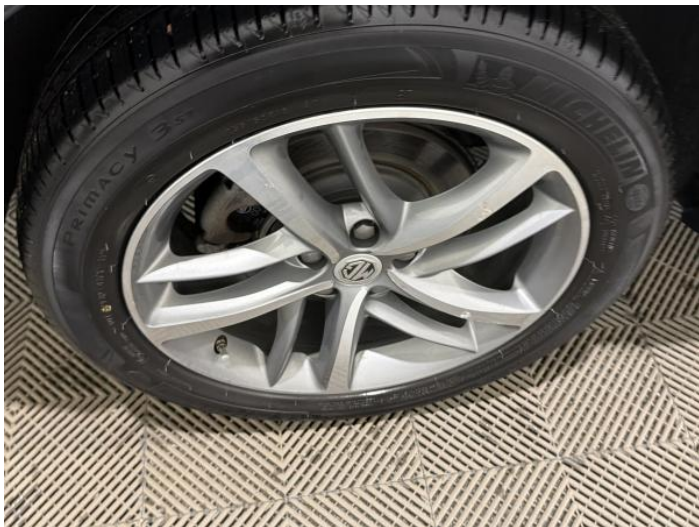
11: Wheel osr Scratched Over 50mm
