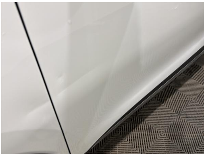
5: Door nsf Dented Over 30mm
