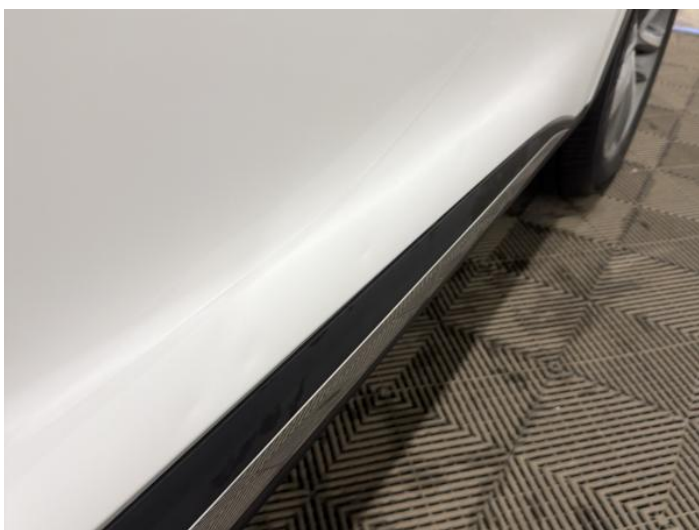
13: Door osf Dented Between 10mm + 30mm
