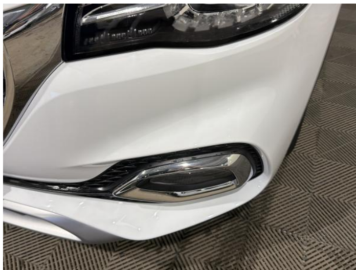
2: Bumper Front Scratched 25 to 100mm Thru Paint
