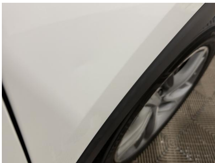
14: Wing osf Dented Between 10mm + 30mm
