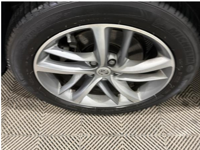
3: Wheel nsf Scratched Up To 50mm
