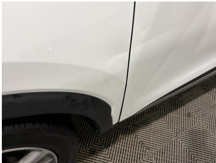
4: Wing nsf Dented Over 30mm
