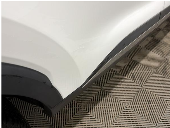
12: Door osr Dented Over 2 UpTo 10mm
