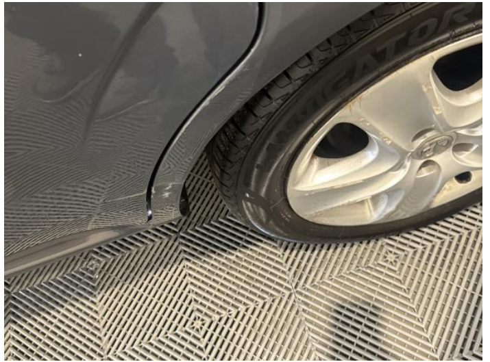
6: Qtr Panel nsr Dented With Paint Damage
