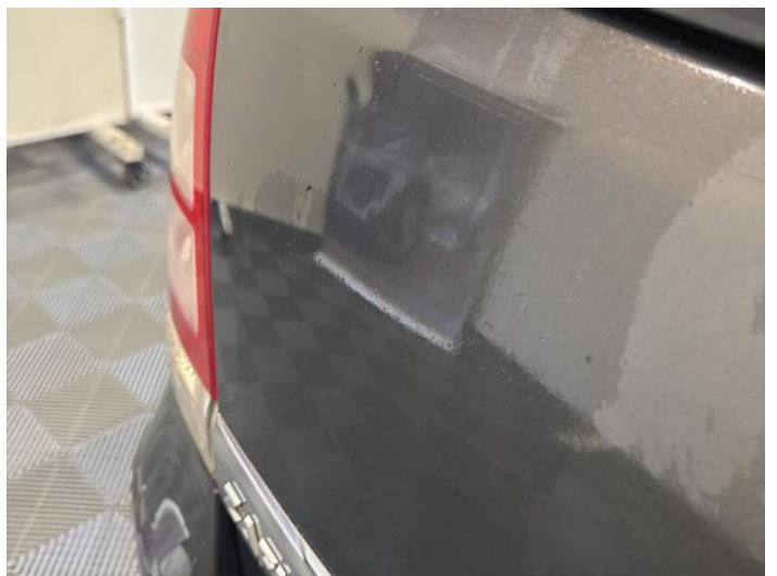
8: Boot Lid Dented Over 2 UpTo 10mm
