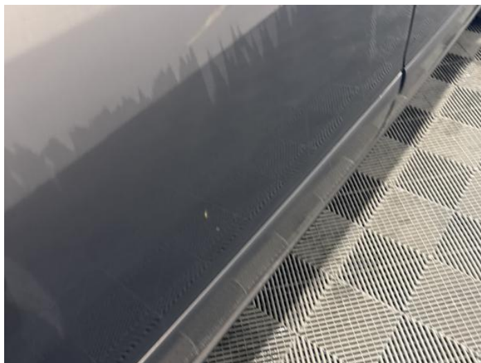
10: Door osr Scratched Over 25mm Thru Paint
