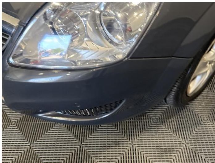
2: Bumper Front Chipped Multiple Chips
