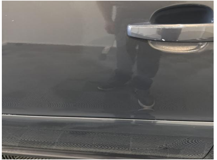
4: Door nsf Dented With Paint Damage
