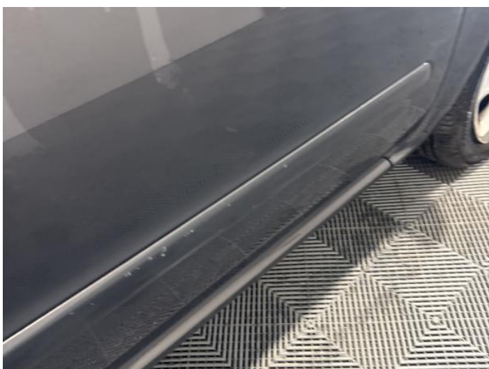
11: Door osf Chipped Multiple Chips
