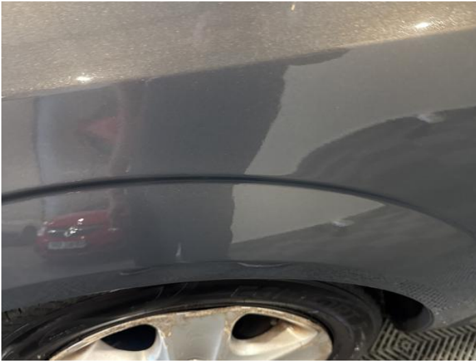
3: Wing nsf Dented Over 2 UpTo 10mm
