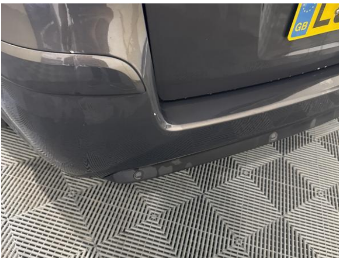
7: Bumper Rear Scratched Over 100mm Thru Paint
