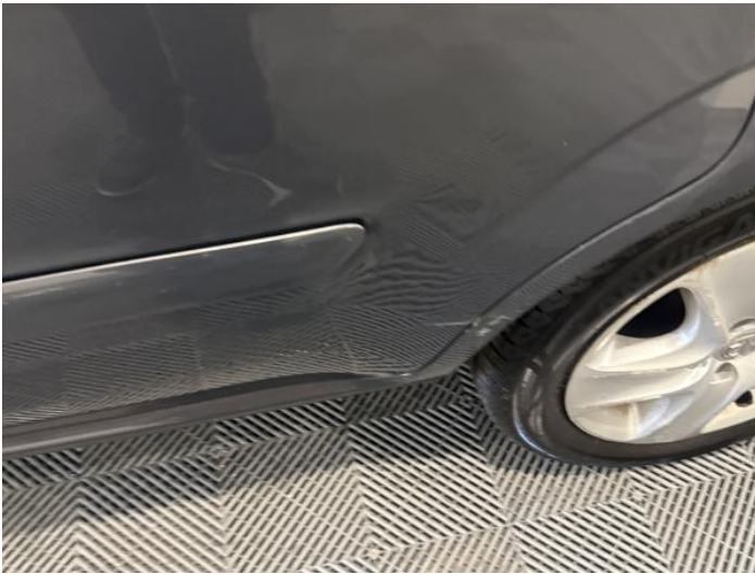
5: Door nsr Dented With Paint Damage
