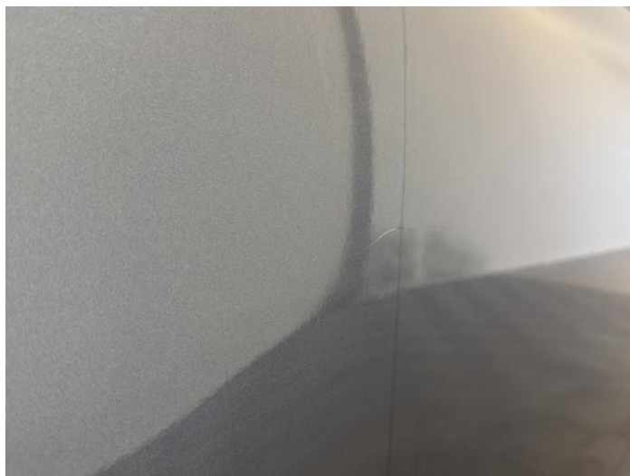
16: Door osr Scratched UpTo 25mm Thru Paint
