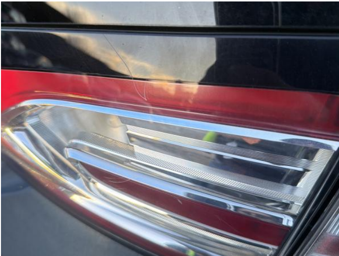
23: Lamp osr Broken Replace
