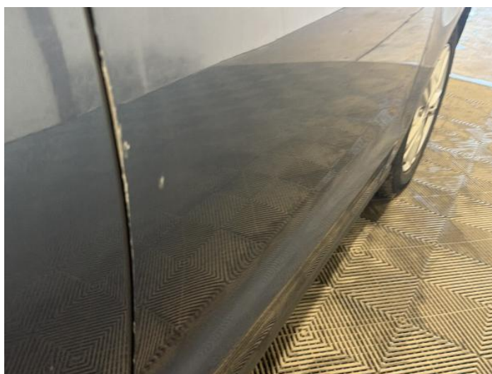
18: Door osf Scratched Over 25mm Thru Paint
