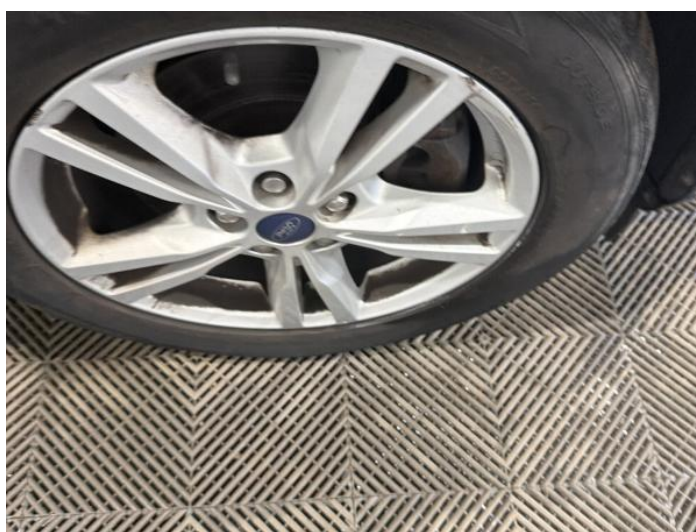
20: Wheel osf Scratched Over 50mm
