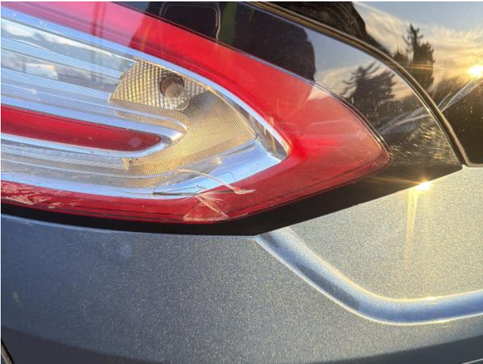
22: Lamp nsr Broken Replace
