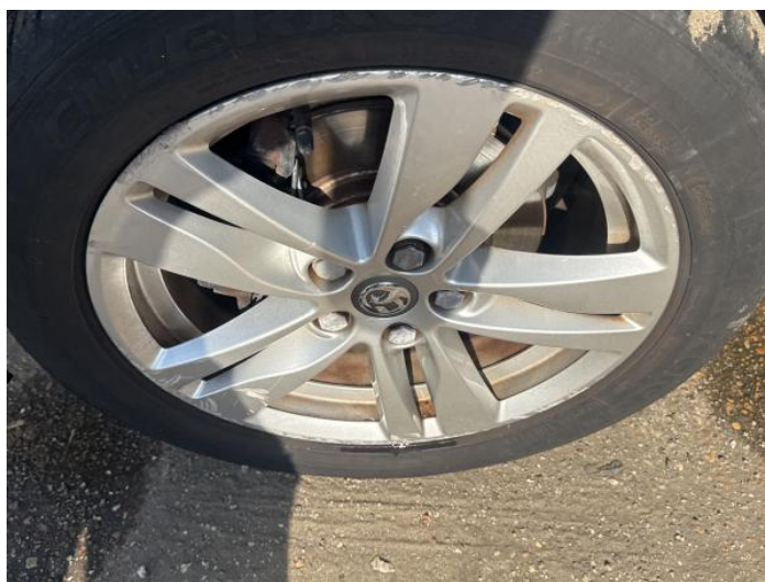
8: Wheel nsf Scratched Over 50mm
