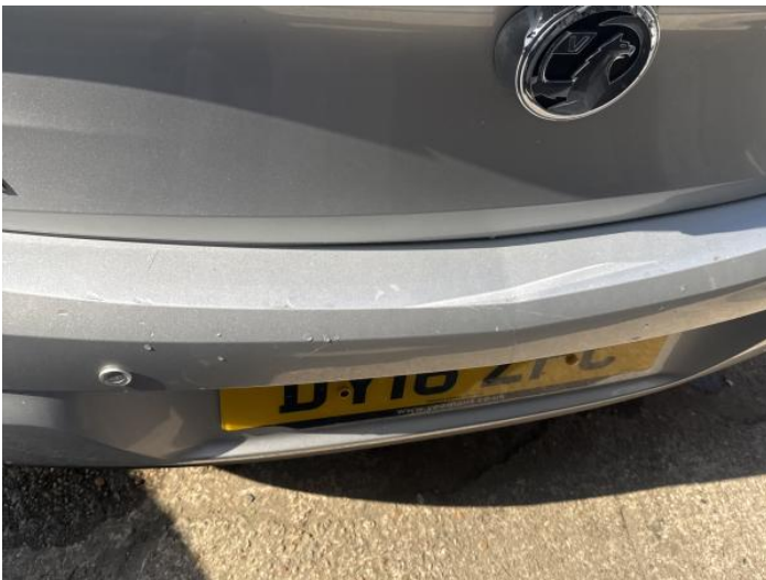
1: Bumper Rear Scratched 25 to 100mm Thru Paint
