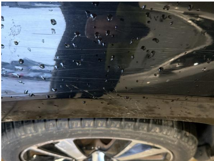
3: Wing nsf Dented Over 2 UpTo 10mm
