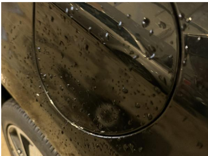
9: Qtr Panel nsr Dented Over 2 UpTo 10mm
