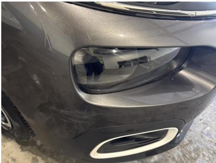
9: Bumper Front Scratched 25 to 100mm Thru Paint
