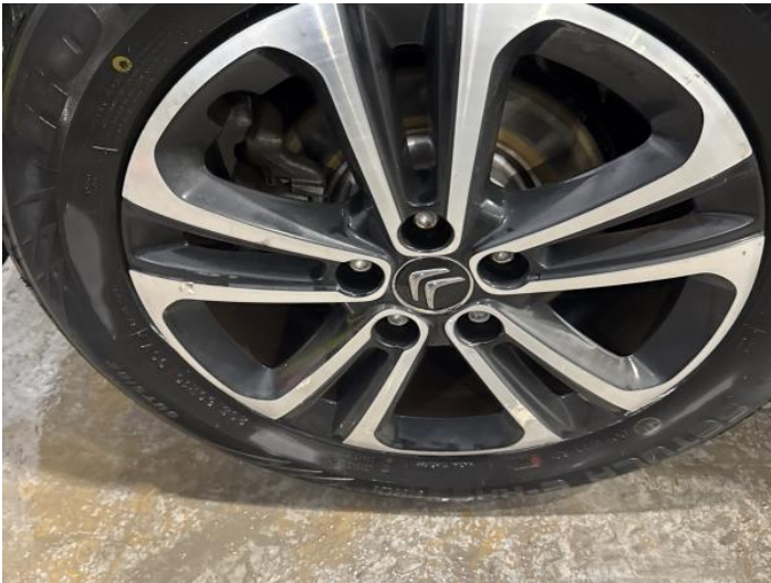
5: Wheel osr Scratched Over 50mm
