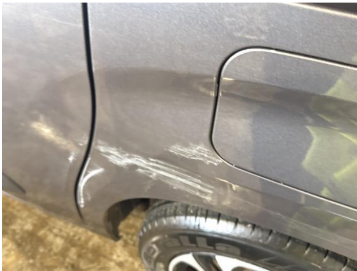
15: Qtr Panel nsr Dented With Paint Damage
