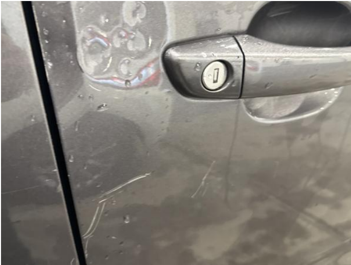
3: Door osf Dented With Paint Damage
