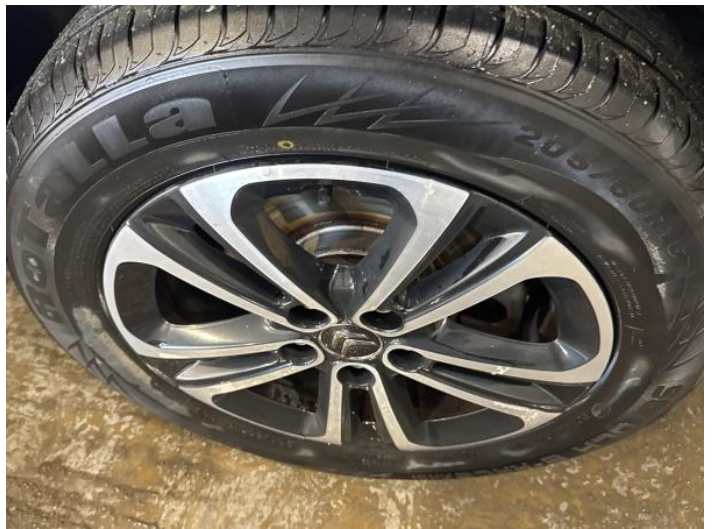
16: Wheel nsr Scratched Over 50mm
