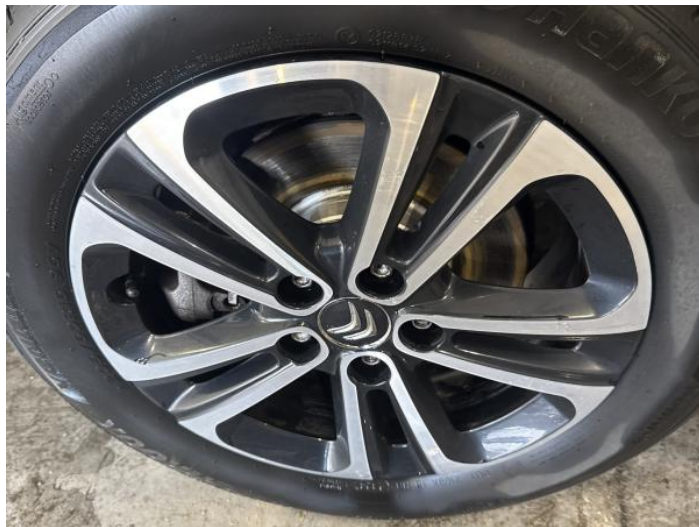
12: Wheel nsf Scratched Up To 50mm
