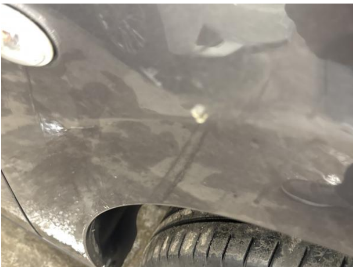
7: Wing osf Scratched Over 25mm Thru Paint
