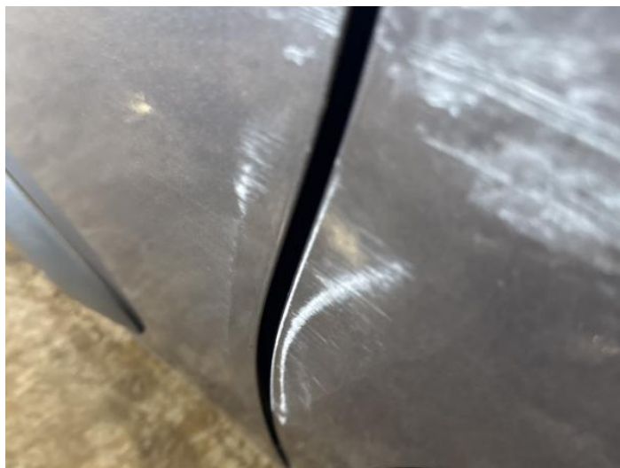
14: Door osf Dented With Paint Damage
